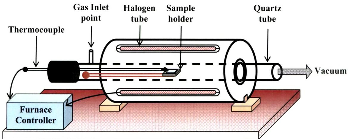
Figure 5.8: Schematic of vacuum based rapid thermal annealing (RTA) furnace [147].
