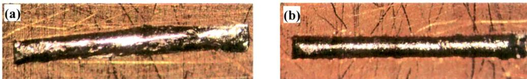
**Figure 5.13: The photograph shows effect of flux applied on melting of Indium preform. (a) While melting 'In' without flux application only shrink and don't show adhesion, on the other hand (b) 'In' melted with flux applied shows uniform melting and better adhesion to the substrate.**
