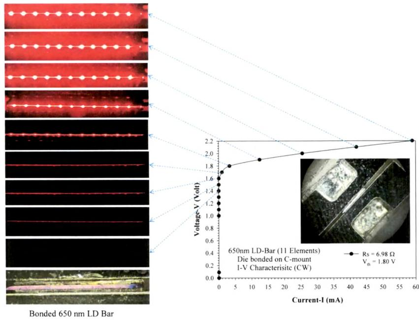
Figure 5.18: CW I-V characteristics and luminescence at different electrical power from the 650 nm laser diode bar package module (illustrated in inset photograph).
