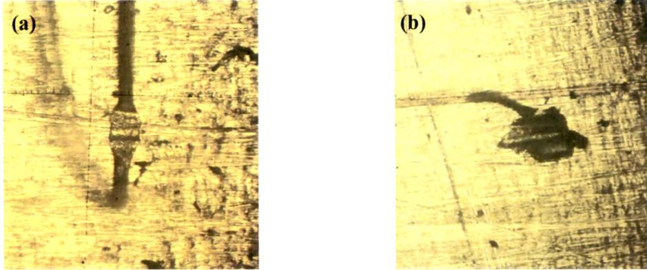
**Figure 5.12: Wedge bond foot prints under microscope: (a) Optimized bond, and (b) Failed bond due to excess ultrasonic power, which results in bond neck-break.**
