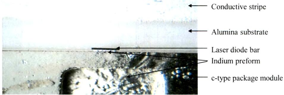
Figure 5.7: 650 nm laser diode bar bonded on c-type package with indium preform. The base for the bonding of this module is alumina substrate with conductive stripe.
