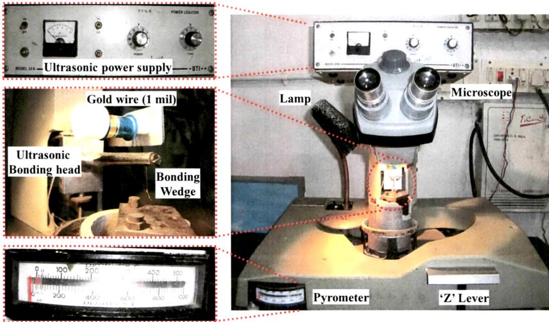
Figure 5.9: K & S make universal ultrasonic wire bonder.
