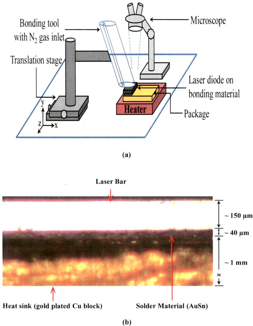
**Figure 5.6: (a) The schematic diagram of the experimental setup of the self assembled manual die bonder. (b) p-side up die-bonding configuration of the 980 nm InGaAs/GaAs ridge waveguide laser diode bar.**
