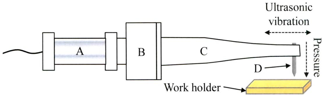
**Figure 5.3:** Typical ultrasonic transducer used for manual wire-bonding: (A) the ultrasonic transducer element; (B) the mounting clamp, which is located on a vibration node and is clamped to the bonding machine; (C) referred to as the horn (tapered to amplify the ultrasonic wave); (D) the tool/capillary, which is clamped perpendicular to the axis of the horn.
