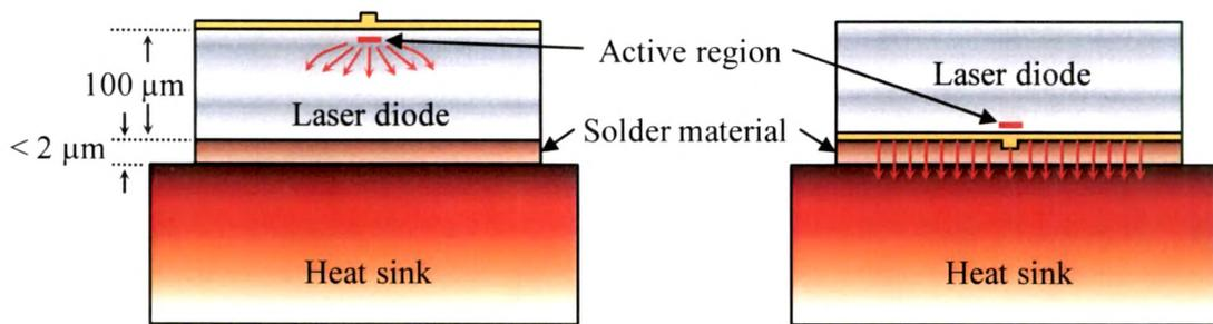
**Figure 5.1: Different bonding configurations of ridge-waveguide laser diodes. (a) For p-side up bonded laser diode, the heat generated in the active region is ineffectively transferred through the substrate; (b) For p-side down bonded laser diode, the heat flux is effectively reached the heat sink within several microns.**
