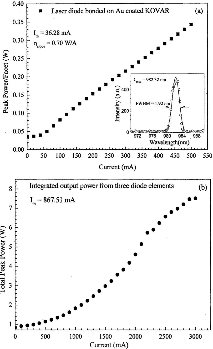
Figure 5.14: (a) Pulse L-I characteristic curve of laser diode elements bonded p-side up with In preform on gold plated KOVAR, inset figure shows typical emission spectrum. (b) Pulse L-I characteristic curve of laser diode bar with three elements bonded p-side down configuration.
