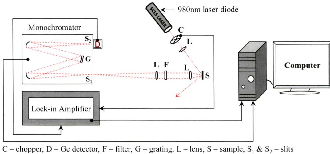
**Figure 6.15: Block diagram of Photoluminescence set up.**
