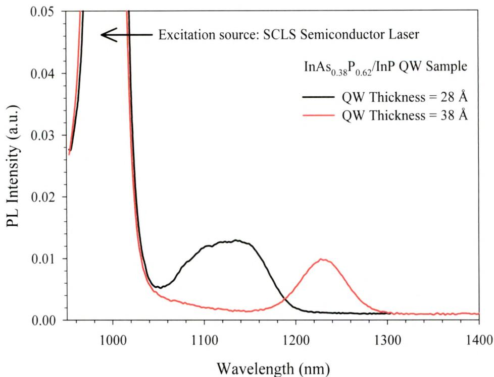
Figure 6.17: PL with 980 nm SCLS Laser
