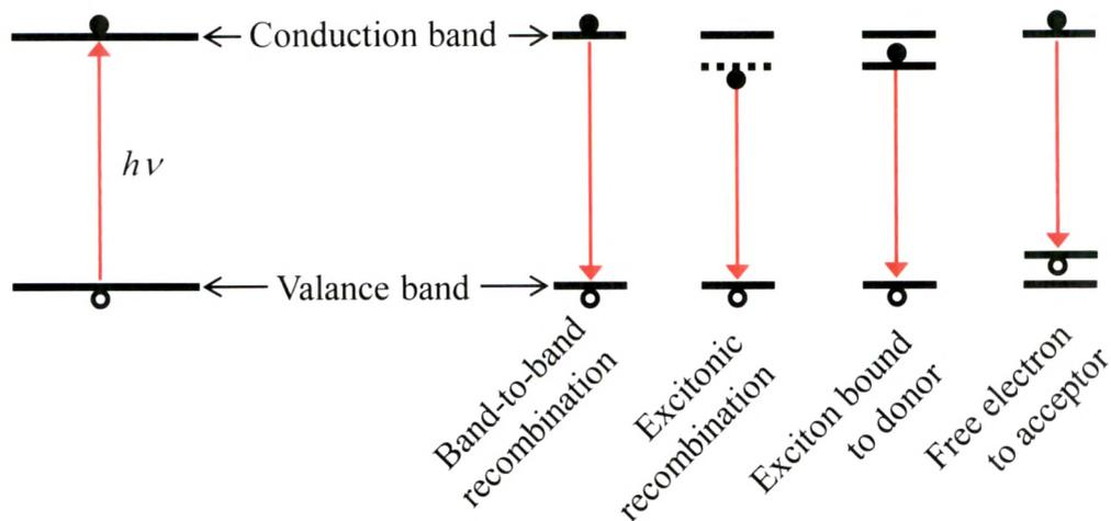
**Figure 6.14: Transition during Photoluminescence. [179]**
