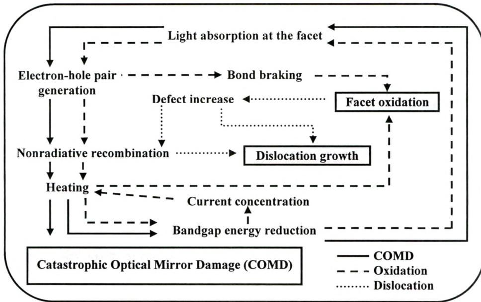
**Figure 6.3: Degradation mechanism in edge-emitting laser diode. This self-destructing cycle of laser diode degradation finally comes to an end with catastrophic optical mirror damage (COMD). [163, 164]**
