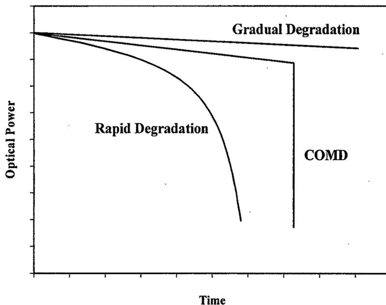
**Figure 6.2: Various degradation modes of laser diode.**
