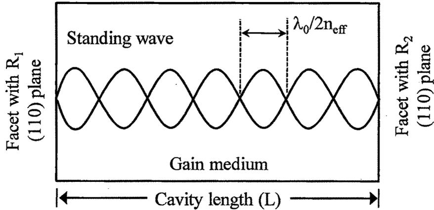
Figure 1.7: Illustration of standing wave in a Fabry-Perot resonator.
