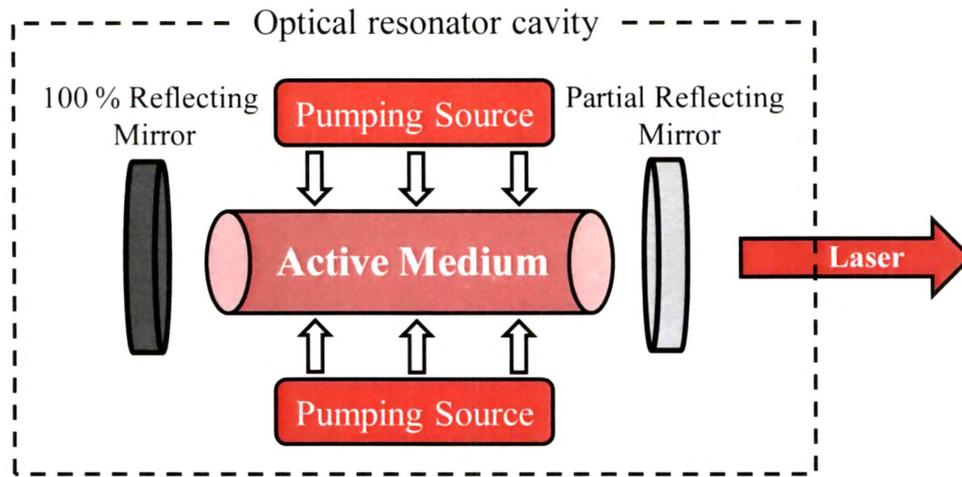
Figure 1.2: Illustration of basic structure of laser system.
