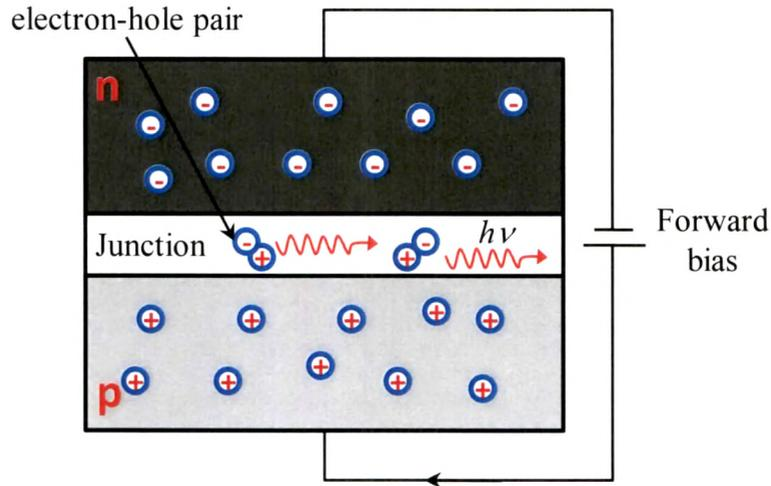
**Figure 1.5: p-n junction under forward bias condition.**
