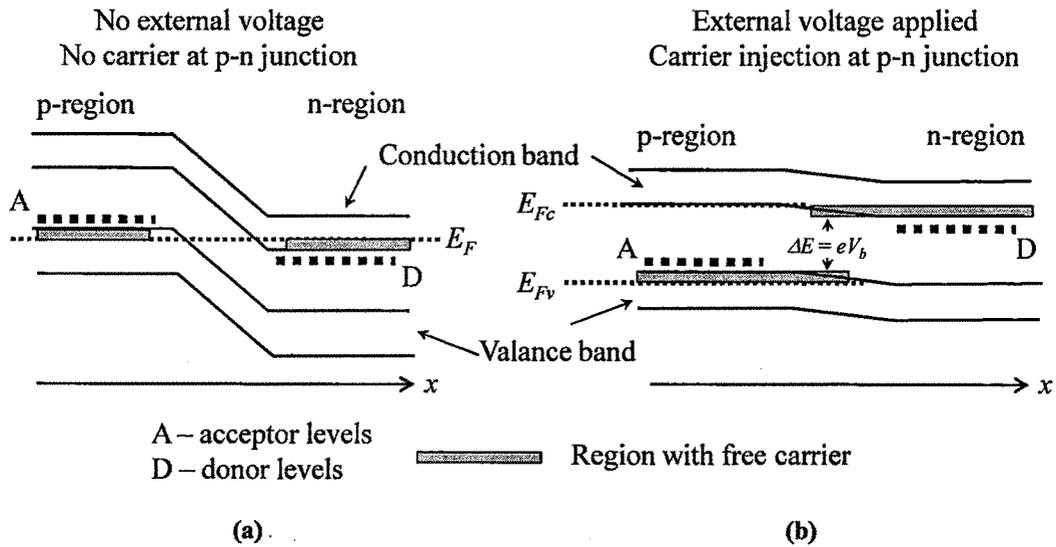
Figure 1.6: Band diagram of p-n junction under (a) zero bias and (b) forward bias conditions.
