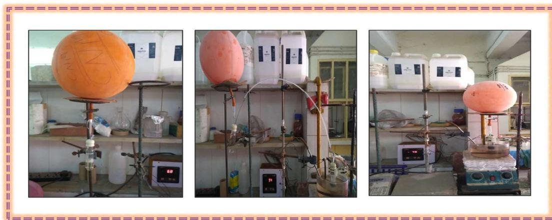
**Figure 2.1** Laboratory setup for the ATRP system.
