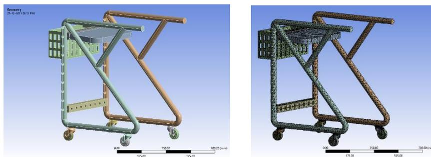
Figure 7.32: Static structural FEA model
