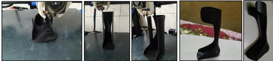
Figure 7.16: 3D printed AFO part
