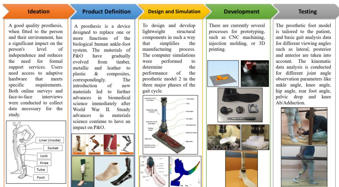
Figure 8.8: Development and testing process for a novel prosthetic foot
