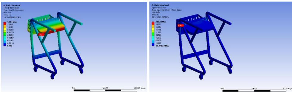
Fig. 29. Total deformation and Equivalent stress for weight of adult as 50 kg in a sitting position (Carbon fiber Composite Material)
