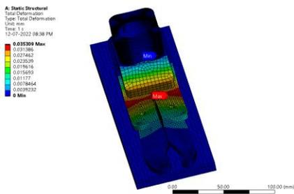
Figure 199: Total deformation (mm)
