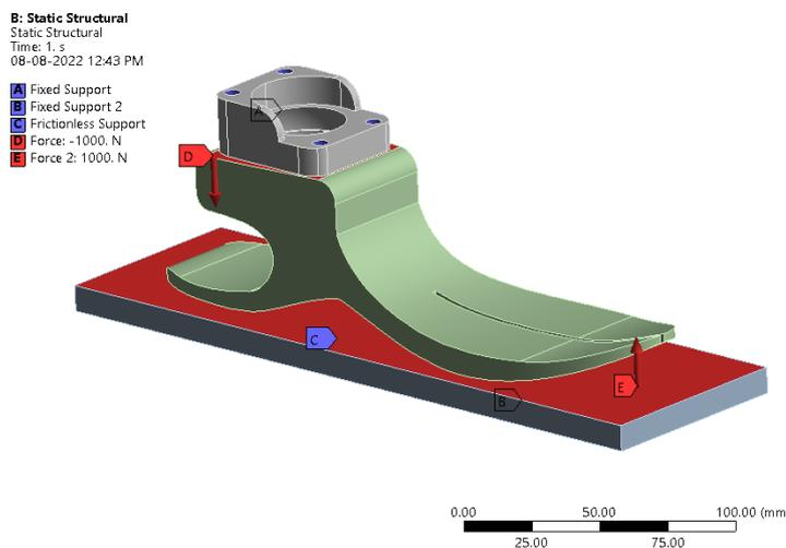
Figure 123: Static structural simulation
