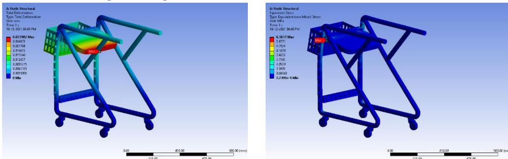
Fig. 1. Total deformation and Equivalent stress for weight of child as 20 kg in a sitting position (S.S. Material)
