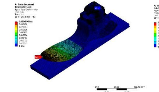
Figure 37: Total deformation (mm)
