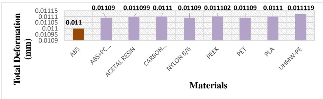
Figure 254: Total deformation in mm for Prosthetic foot model 1 during mid-stance analysis
