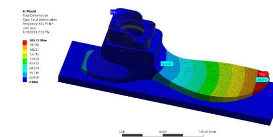
Figure 30: Total deformation (Hz)
