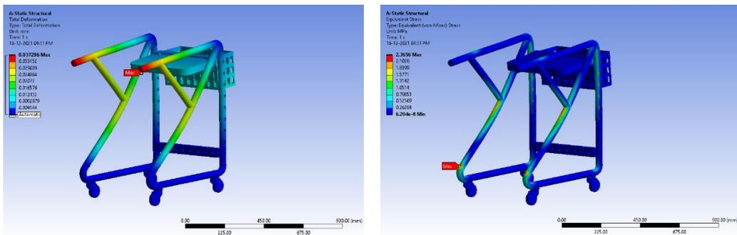
Fig. 2. Total deformation and Equivalent stress for weight of child as 20 kg in standing position (S.S. Material)
