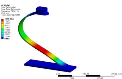
Figure 329: Total deformation (Hz)
