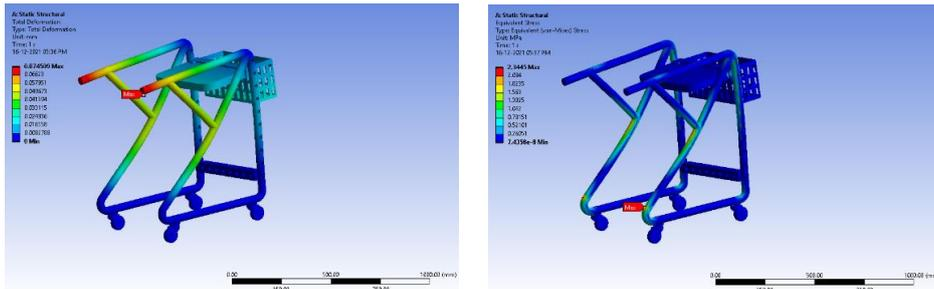
Fig. 10. Total deformation and Equivalent stress for weight of child as 20 kg in standing position (Ti. Material)
