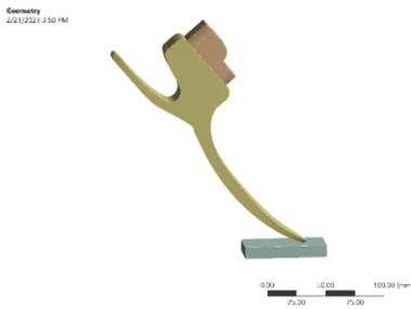
Figure 82: Prosthetic foot geometry
