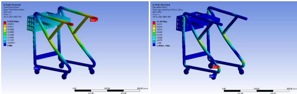
Fig. 24. Total deformation and Equivalent stress for weight of adult as 100 kg in standing position (Al. Material)
