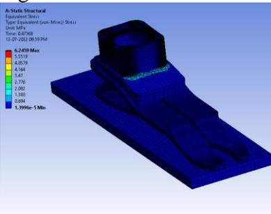
Figure 201: Equivalent Stress
