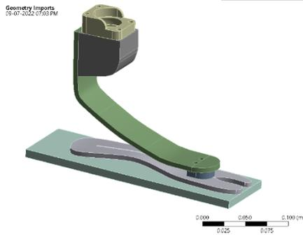
Figure 207: Prosthetic foot geometry
