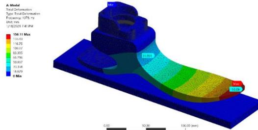
Figure 18: Total deformation (Hz)
