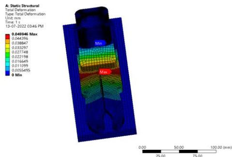
Figure 172: Total deformation (mm)
