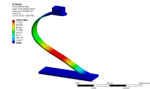
Figure 321: Total deformation (Hz)
