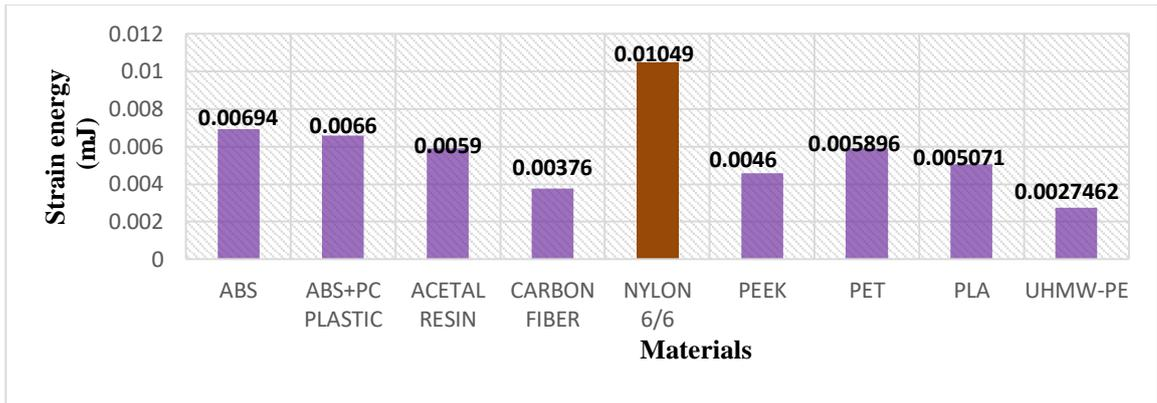
Figure 127: Strain energy for Prosthetic foot model 1 during mid-stance analysis
