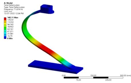
Figure 301: Total deformation (Hz)
