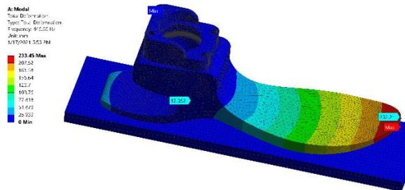
Figure 6: Total deformation (Hz)
