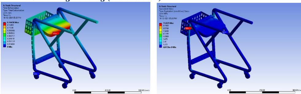
Fig. 7. Total deformation and Equivalent stress for weight of child as 40 kg in a sitting position (Al. Material)
