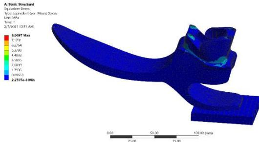
Figure 55: Equivalent Stress
