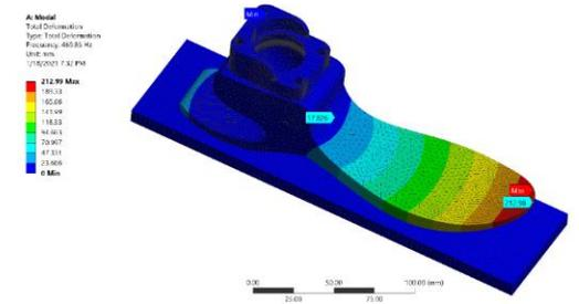
Figure 34: Total deformation (Hz)
