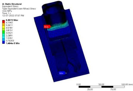
Figure 197: Equivalent Stress
