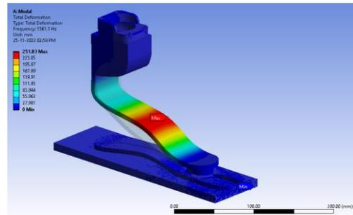
Figure 247: Total deformation (Hz)
