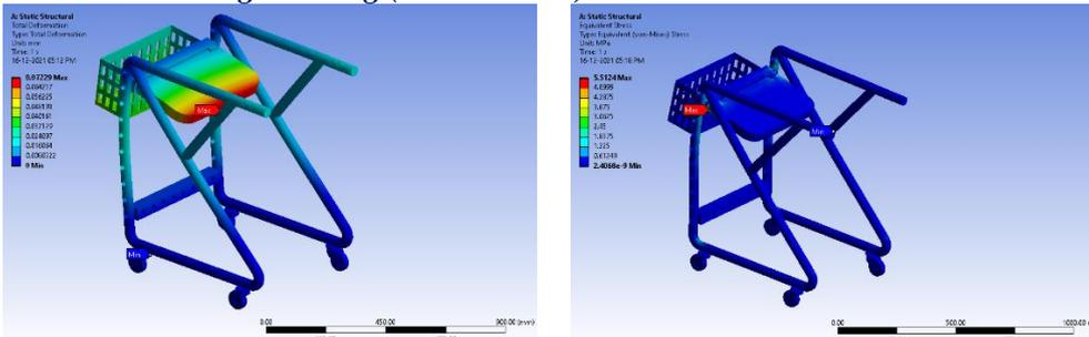
Fig. 5. Total deformation and Equivalent stress for weight of child as 20 kg in a sitting position (Al. Material)
