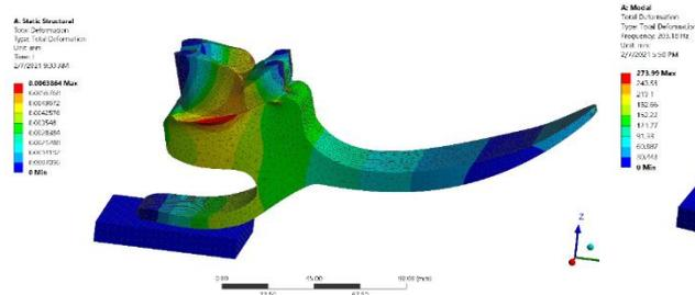
Figure 65: Total deformation (mm)
