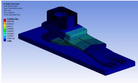
Figure 175: Total deformation (mm)
