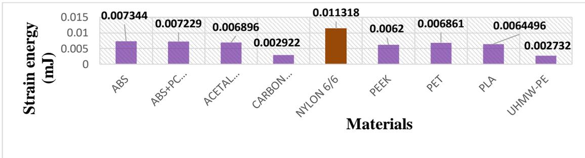
Figure 299: Strain energy for Prosthetic foot model 1 during mid-stance analysis
