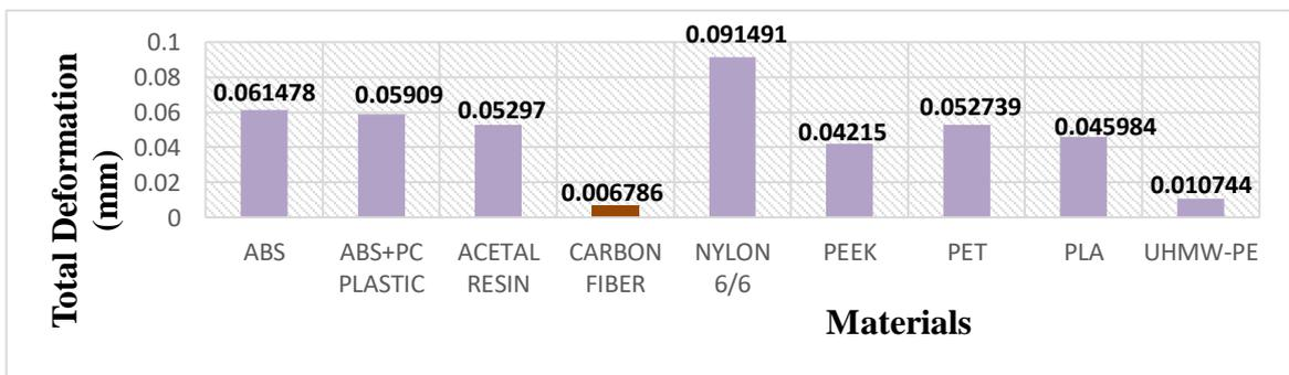
Figure 297: Total deformation in mm for Prosthetic foot model 1 during mid-stance analysis
