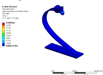
Figure 334: Equivalent Stress
