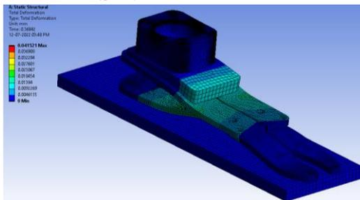
Figure 179: Total deformation (mm)
