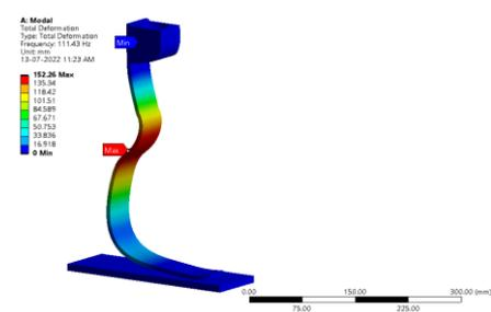
Figure 282: Total deformation (Hz)
