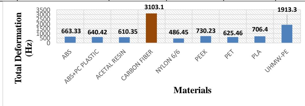
Figure 167: Total deformation in Hz for Prosthetic foot model 1 during mid-stance analysis
