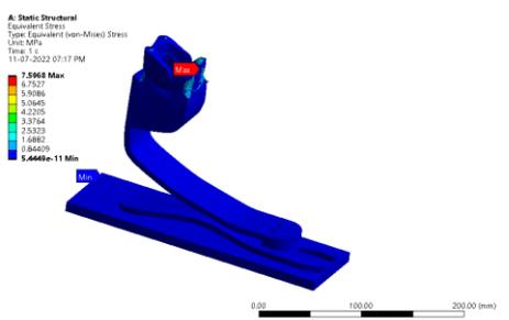
Figure 240: Equivalent Stress
