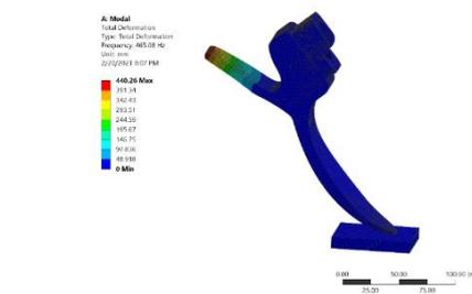
Figure 94: Total deformation (Hz)
