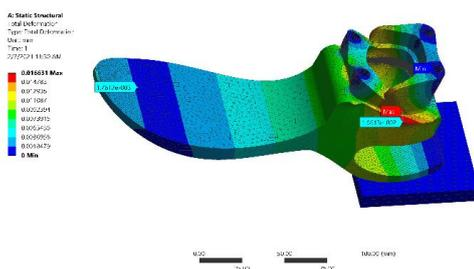
Figure 61: Total deformation (mm)
