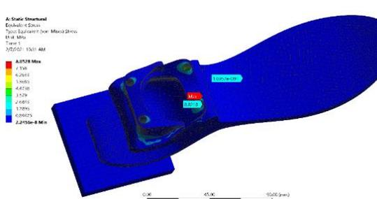
Figure 51: Equivalent Stress
