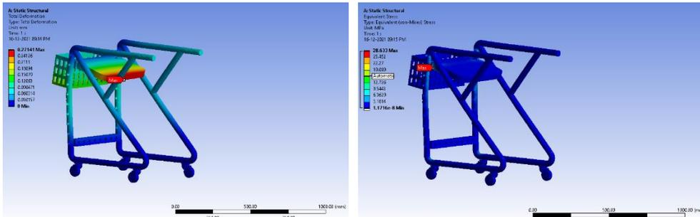
Fig. 27. Total deformation and Equivalent stress for weight of adult as 100 kg in a sitting position (Ti. Material)
