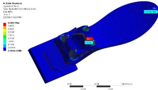
Figure 75: Equivalent Stress
