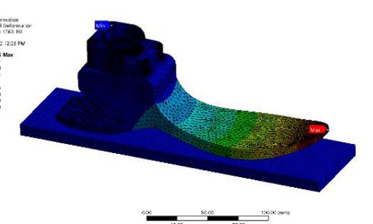
Figure 38: Total deformation (Hz)
