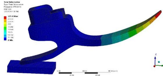
Figure 46: Total deformation (Hz)
