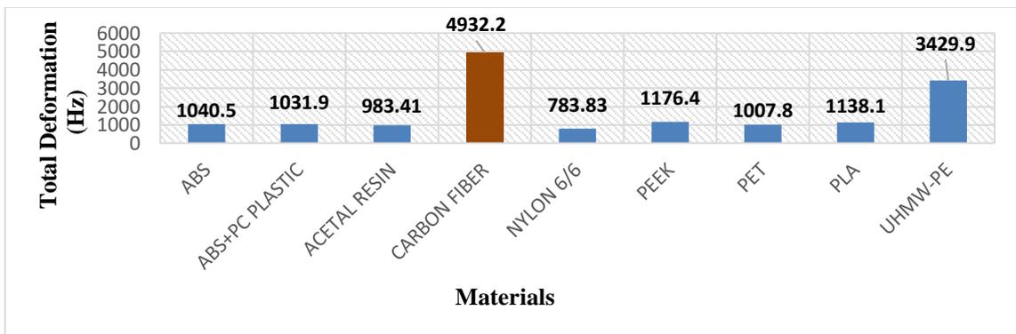
Figure 124: Total deformation in Hz for Prosthetic foot model 1 during mid-stance analysis
