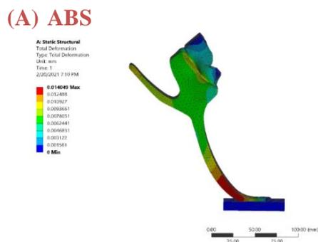
Figure 85: Total deformation (mm)
