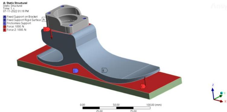
Figure 4: Static structural simulation
