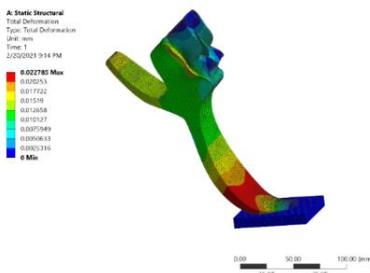
Figure 101: Total deformation (mm)
