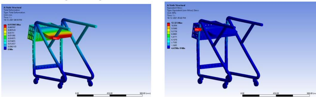
Fig. 3. Total deformation and Equivalent stress for weight of child as 40 kg in a sitting position (S.S. Material)
