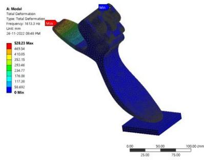
Figure 117: Total deformation (Hz)
