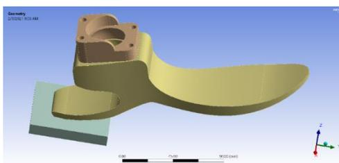
Figure 42: Prosthetic foot geometry
