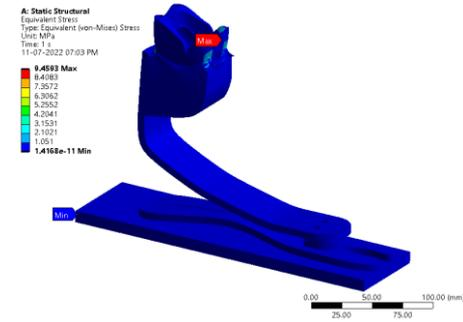
Figure 236: Equivalent Stress
