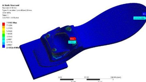
Figure 63: Equivalent Stress
