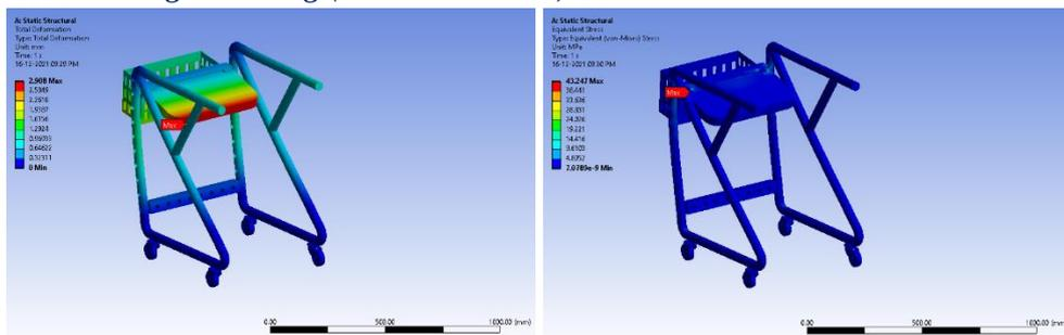
Fig. 31. Total deformation and Equivalent stress for weight of adult as 100 kg in a sitting position (Carbon fiber Composite Material)
