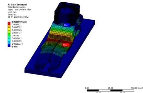
Figure 203: Total deformation (mm)
