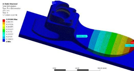
Figure 29: Total deformation (mm)
