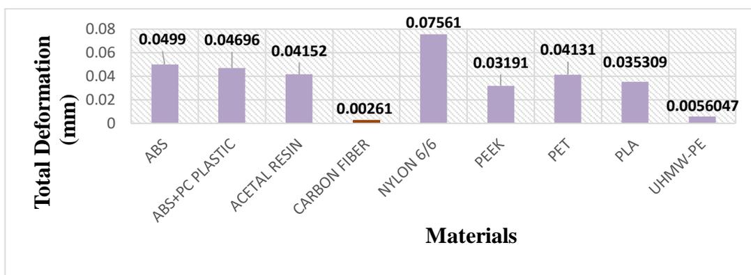
Figure 168: Total deformation in mm for Prosthetic foot model 1 during mid-stance analysis
