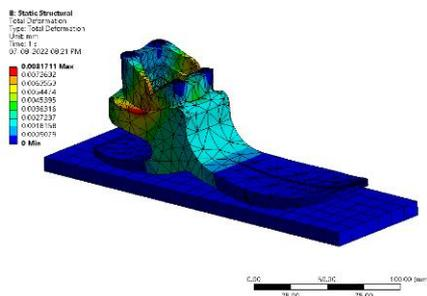
Figure 132: Total deformation (mm)
