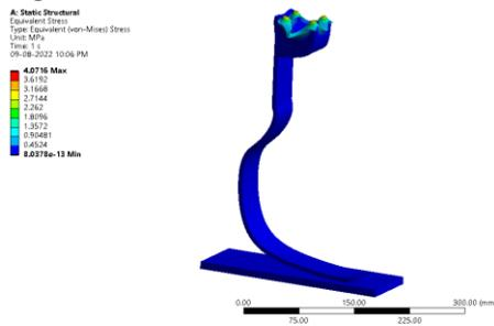
Figure 279: Equivalent Stress
