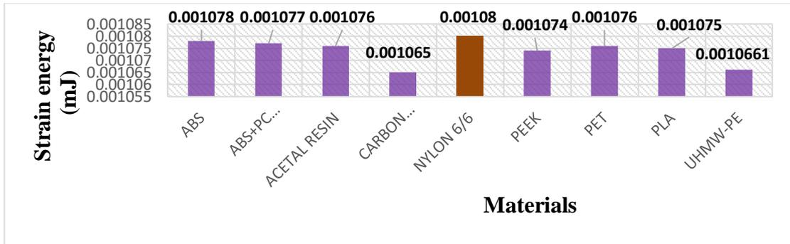
Figure 256: Strain energy for Prosthetic foot model 1 during mid-stance analysis
