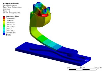
Figure 235: Total deformation (mm)
