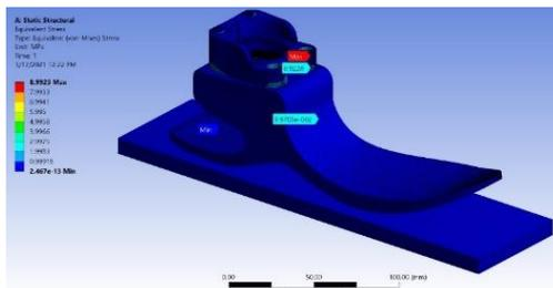
Figure 7: Equivalent Stress
