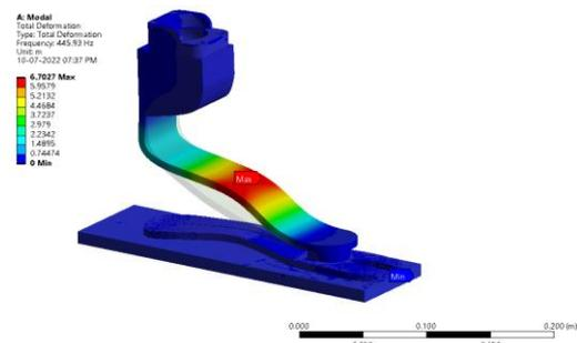
Figure 223: Total deformation (Hz)
