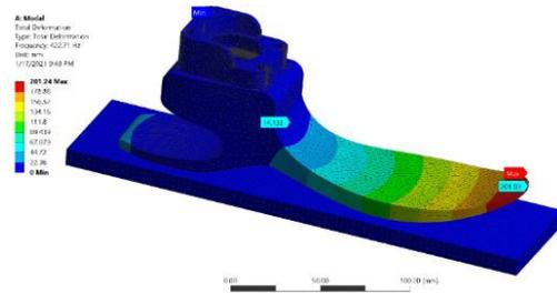
Figure 14: Total deformation (Hz)
