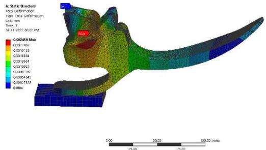
Figure 77: Total deformation (mm)
