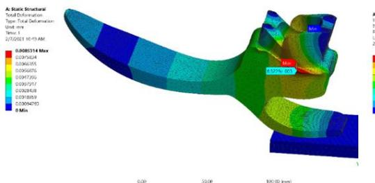
Figure 53: Total deformation (mm)
