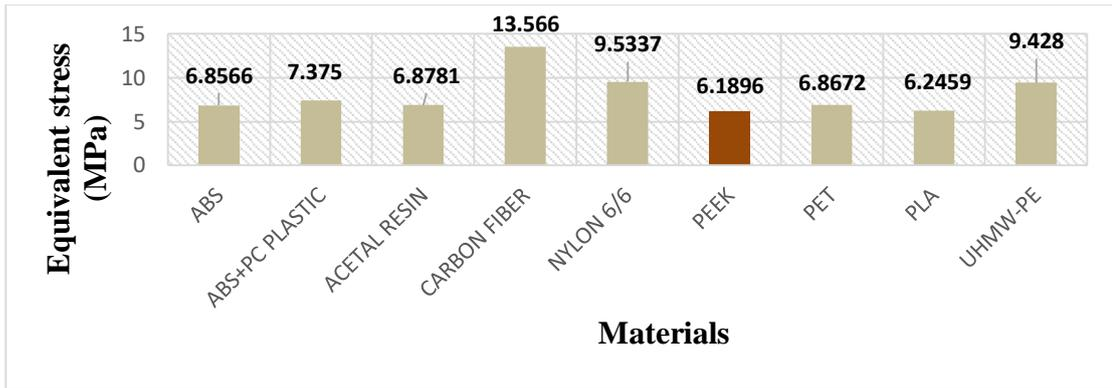
Figure 169: Equivalent stress for Prosthetic foot model 1 during mid-stance analysis
