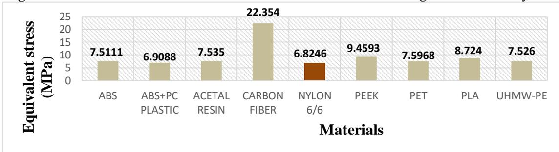
Figure 212: Equivalent stress for Prosthetic foot model 1 during mid-stance analysis
