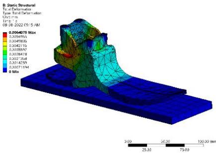
Figure 148: Total deformation (mm)
