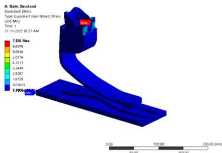
Figure 248: Equivalent Stress
