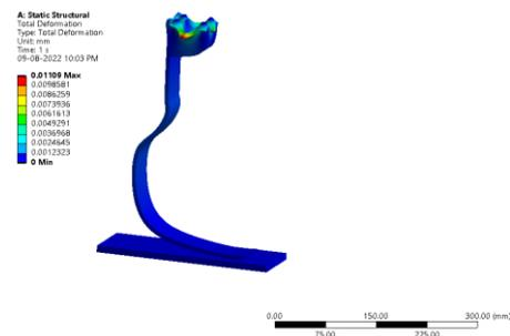
Figure 273: Total deformation (mm)
