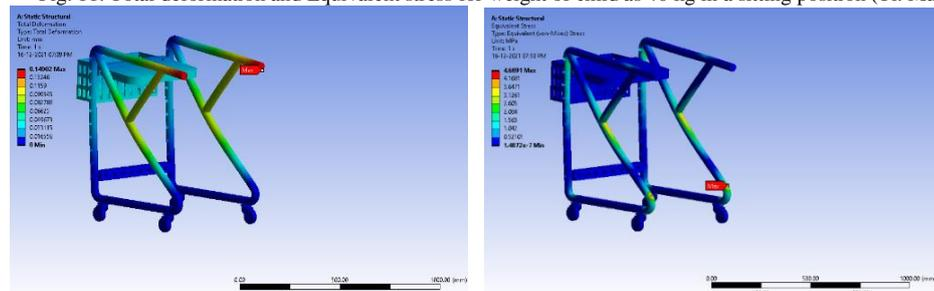
Fig. 12. Total deformation and Equivalent stress for weight of child as 40 kg in standing position (Ti. Material)
