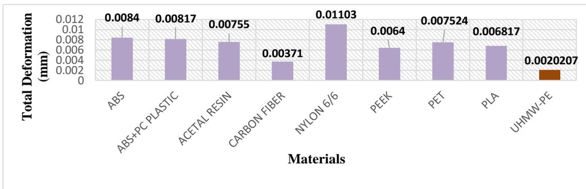
Figure 125: Total deformation in mm for Prosthetic foot model 1 during mid-stance analysis
