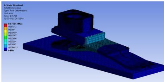
Figure 187: Total deformation (mm)
