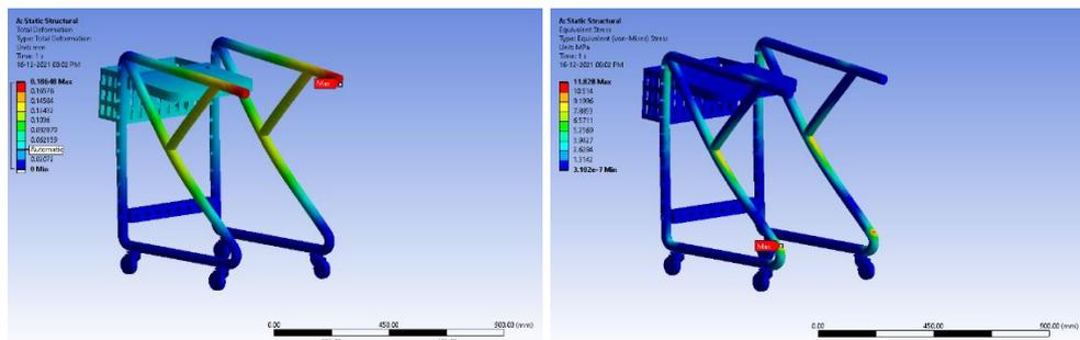
Fig. 20. Total deformation and Equivalent stress for weight of adult as 100 kg in standing position (S.S. Material)
