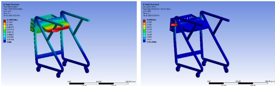
Fig. 19. Total deformation and Equivalent stress for weight of adult as 100 kg in a sitting position (S.S. Material)
