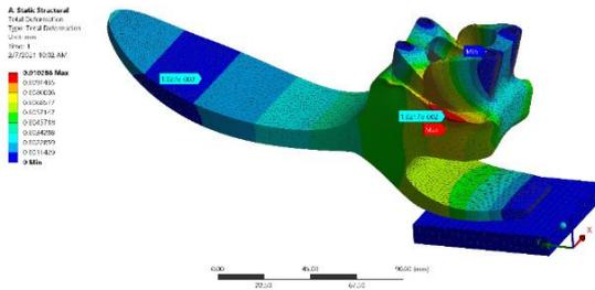
Figure 45: Total deformation (mm)
