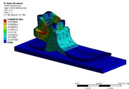
Figure 128: Total deformation (mm)
