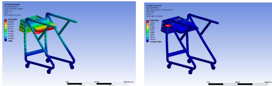
Fig. 13. Total deformation and Equivalent stress for weight of child as 20 kg in a sitting position (Carbon fiber Composite Material)
