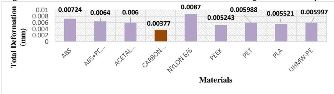
Figure 211: Total deformation in mm for Prosthetic foot model 1 during mid-stance analysis
