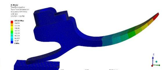
Figure 50: Total deformation (Hz)
