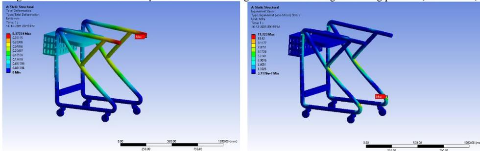
Fig. 28. Total deformation and Equivalent stress for weight of adult as 100 kg in standing position (Ti. Material)
