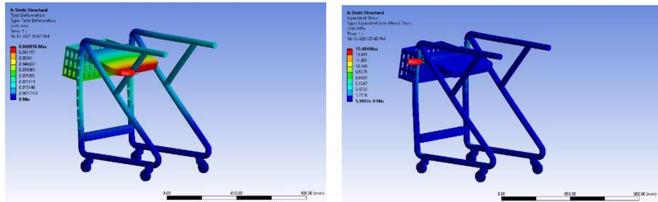
Fig. 17. Total deformation and Equivalent stress for weight of adult as 50 kg in a sitting position (S.S. Material)
