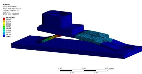
Figure 176: Total deformation (Hz)
