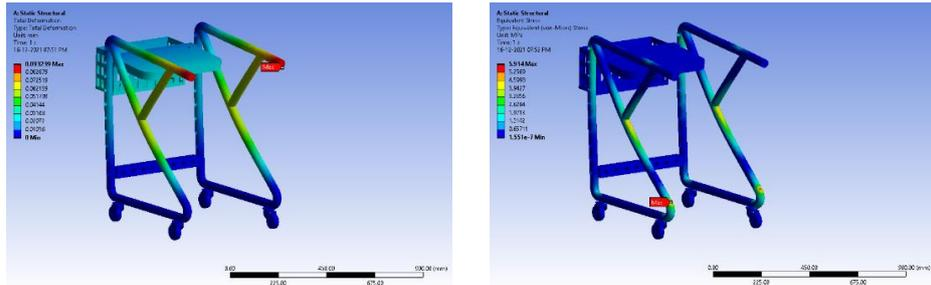
Fig. 18. Total deformation and Equivalent stress for weight of adult as 50 kg in standing position (S.S. Material)
