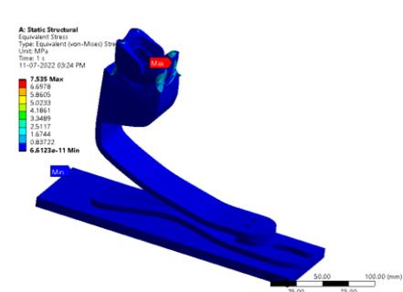
Figure 224: Equivalent Stress
