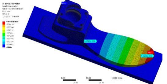
Figure 33: Total deformation (mm)
