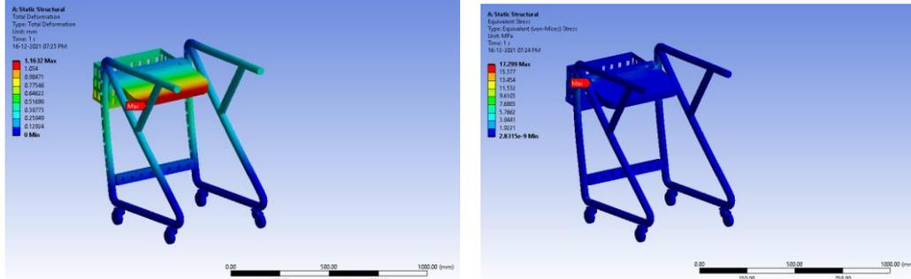
Fig. 15. Total deformation and Equivalent stress for weight of child as 40 kg in a sitting position (Carbon fiber Composite Material)
