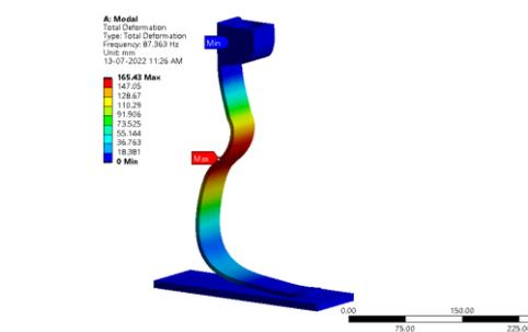
Figure 274: Total deformation (Hz)
