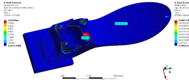
Figure 67: Equivalent Stress
