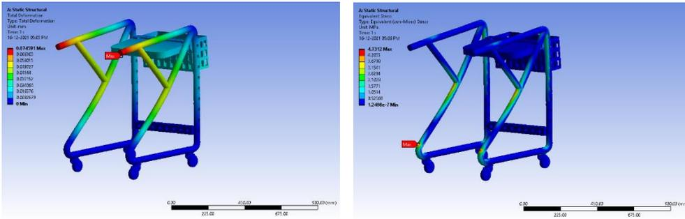
Fig. 4. Total deformation and Equivalent stress for weight of child as 40 kg in standing position (S.S. Material)
