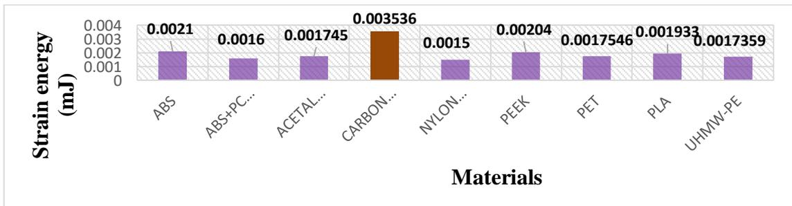
Figure 213: Strain energy for Prosthetic foot model 1 during mid-stance analysis
