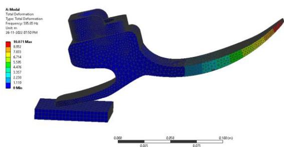
Figure 78: Total deformation (Hz)
