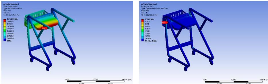
Fig. 9. Total deformation and Equivalent stress for weight of child as 20 kg in a sitting position (Ti. Material)
