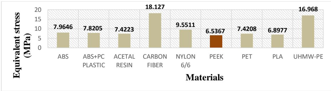
Figure 298: Equivalent stress for Prosthetic foot model 1 during mid-stance analysis
