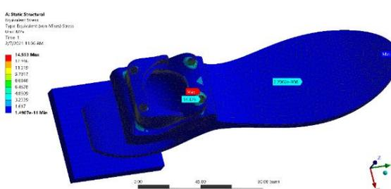
Figure 59: Equivalent Stress
