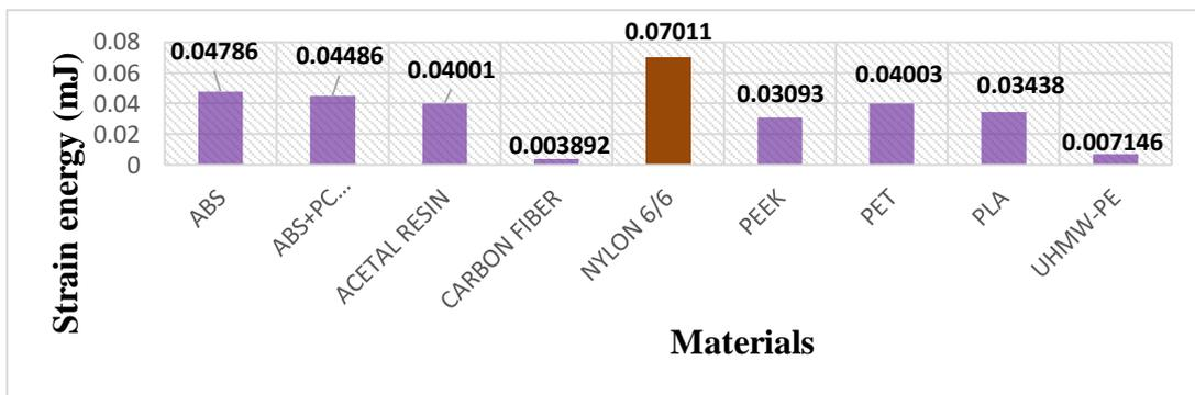
Figure 170: Strain energy for Prosthetic foot model 1 during mid-stance analysis
