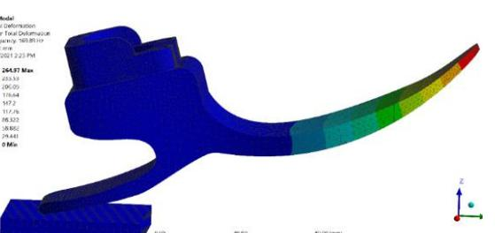
Figure 54: Total deformation (Hz)
