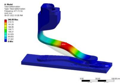
Figure 215: Total deformation (Hz)
