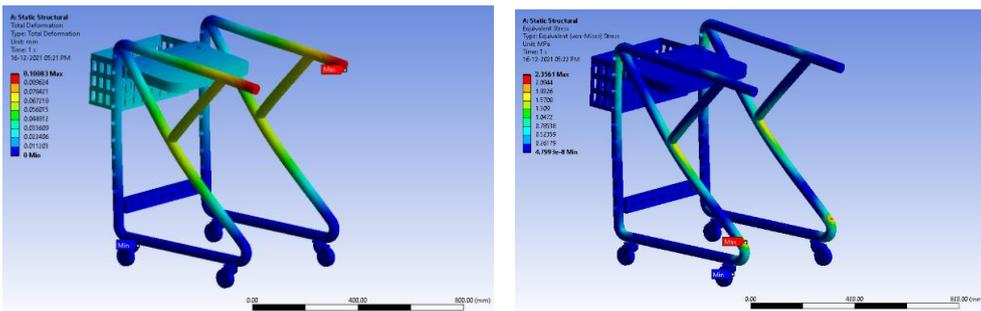
Fig. 6. Total deformation and Equivalent stress for weight of child as 20 kg in standing position (Al. Material)
