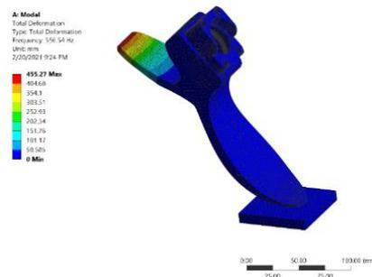
Figure 106: Total deformation (Hz)
