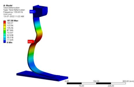
Figure 286: Total deformation (Hz)
