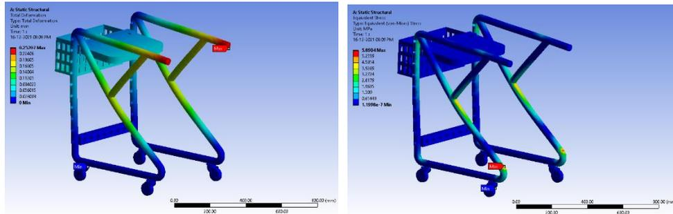
Fig. 22. Total deformation and Equivalent stress for weight of adult as 50 kg in standing position (Al. Material)
