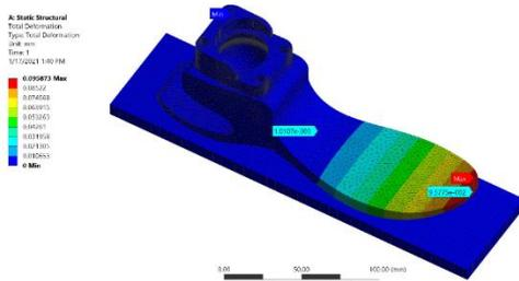
Figure 13: Total deformation (mm)
