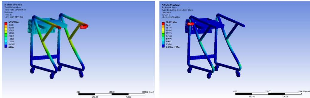
Fig. 32. Total deformation and Equivalent stress for weight of adult as 100 kg in standing position (Carbon fiber Composite Material)
