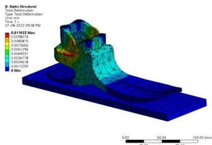
Figure 144: Total deformation (mm)
