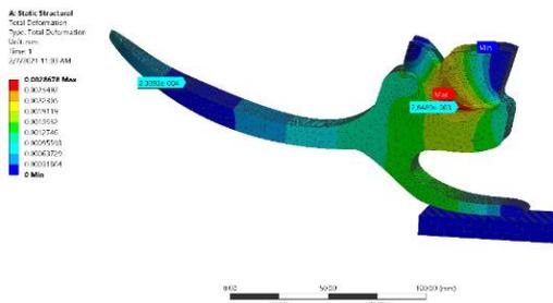
Figure 57: Total deformation (mm)
