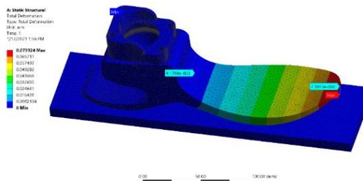
Figure 17: Total deformation (mm)
