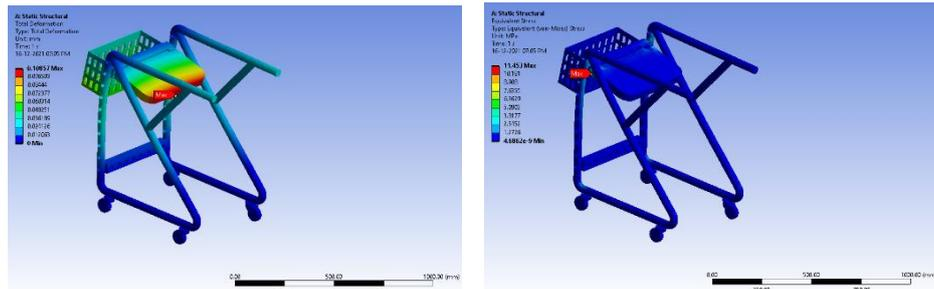
Fig. 11. Total deformation and Equivalent stress for weight of child as 40 kg in a sitting position (Ti. Material)
