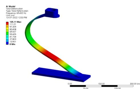
Figure 325: Total deformation (Hz)
