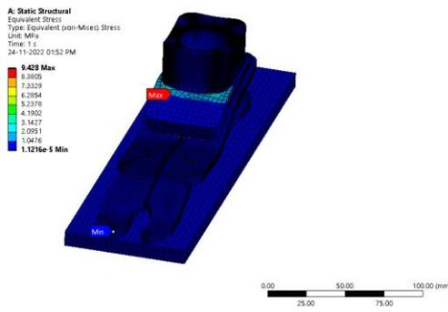
Figure 205: Equivalent Stress
