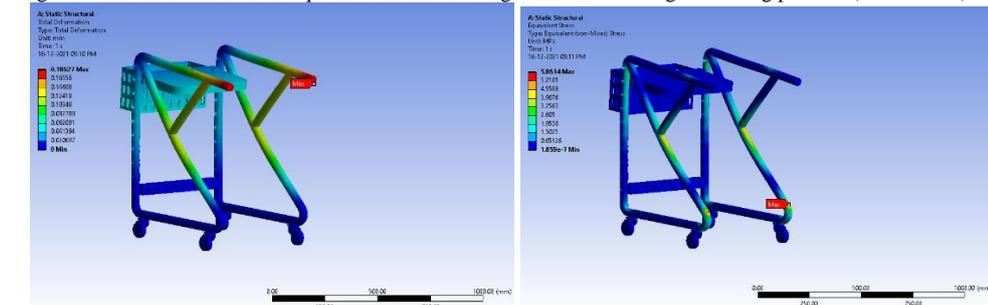
Fig. 26. Total deformation and Equivalent stress for weight of adult as 50 kg in standing position (Ti. Material)
