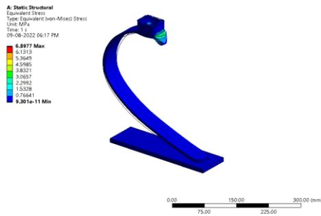
Figure 330: Equivalent Stress
