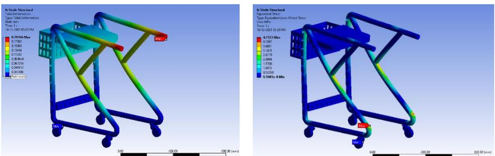
Fig. 8. Total deformation and Equivalent stress for weight of child as 40 kg in standing position (Al. Material)
