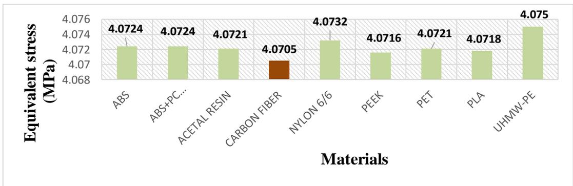
Figure 255: Equivalent stress for Prosthetic foot model 1 during mid-stance analysis
