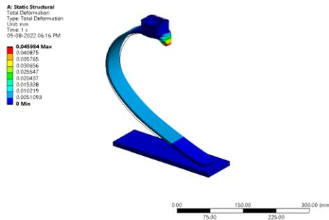
Figure 328: Total deformation (mm)
