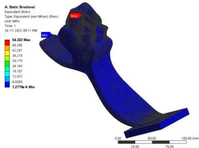
Figure 119: Equivalent Stress
