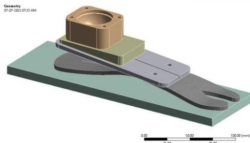
Figure 164: Prosthetic foot geometry
