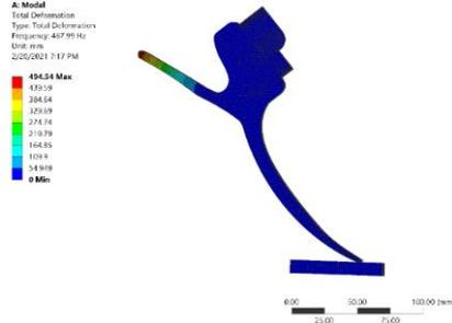
Figure 90: Total deformation (Hz)
