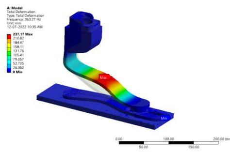
Figure 231: Total deformation (Hz)
