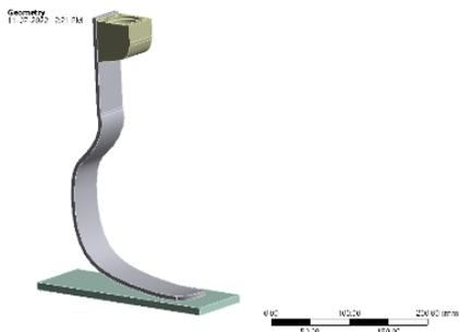
Figure 250: Prosthetic foot geometry
