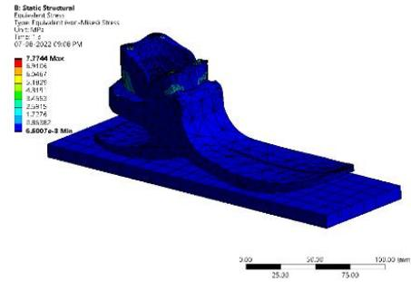
Figure 146: Equivalent Stress
