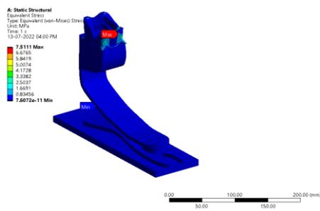
Figure 216: Equivalent Stress
