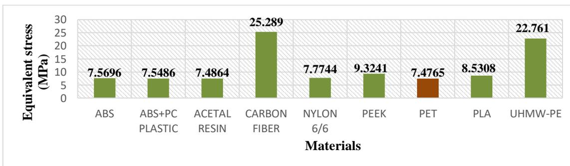
Figure 126: Equivalent stress for Prosthetic foot model 1 during mid-stance analysis
