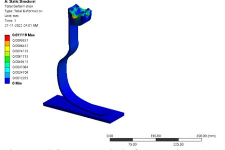
Figure 289: Total deformation (mm)
