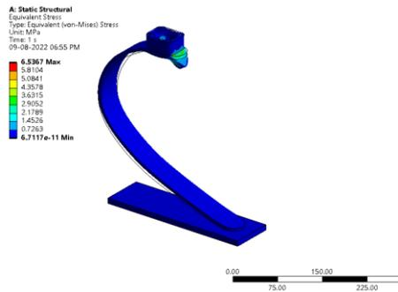
Figure 322: Equivalent Stress
