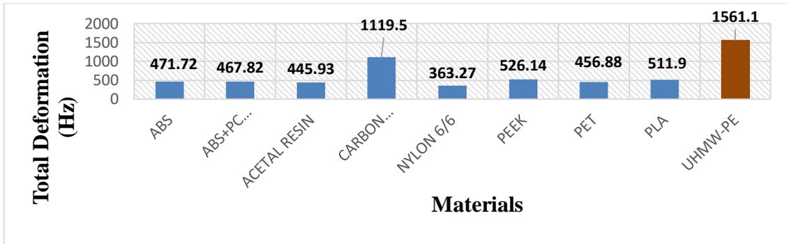
Figure 210: Total deformation in Hz for Prosthetic foot model 1 during mid-stance analysis
