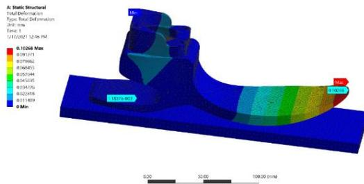
Figure 21: Total deformation (mm)
