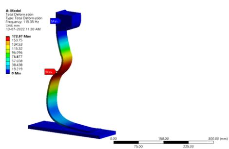
Figure 258: Total deformation (Hz)
