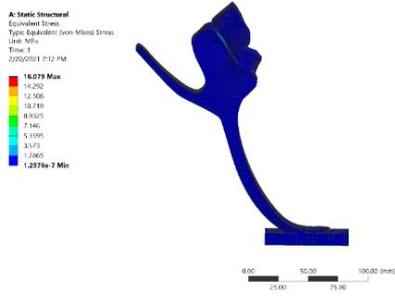
Figure 87: Equivalent Stress
