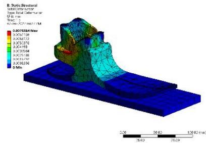
Figure 136: Total deformation (mm)
