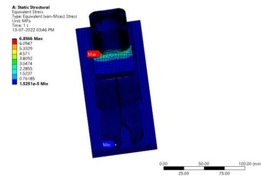
Figure 173: Equivalent Stress
