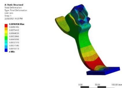
Figure 114: Total deformation (mm)
