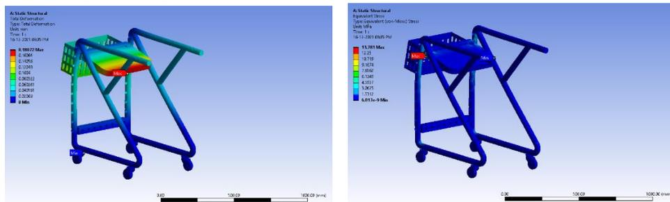
Fig. 21. Total deformation and Equivalent stress for weight of adult as 50 kg in a sitting position (Al. Material)
