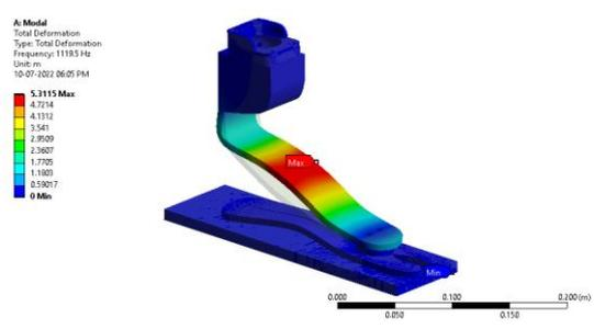
Figure 227: Total deformation (Hz)
