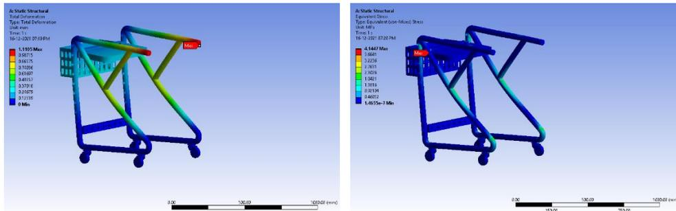
Fig. 14. Total deformation and Equivalent stress for weight of child as 20 kg in standing position (Carbon fiber Composite Material)
