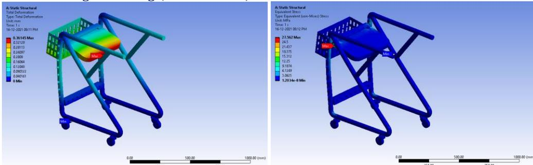
Fig. 23. Total deformation and Equivalent stress for weight of adult as 100 kg in a sitting position (Al. Material)
