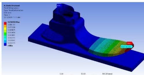
Figure 9: Total deformation (mm)
