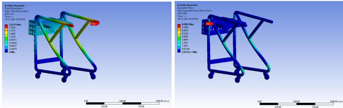
Fig. 16. Total deformation and Equivalent stress for weight of child as 40 kg in standing position (Carbon fiber Material)
