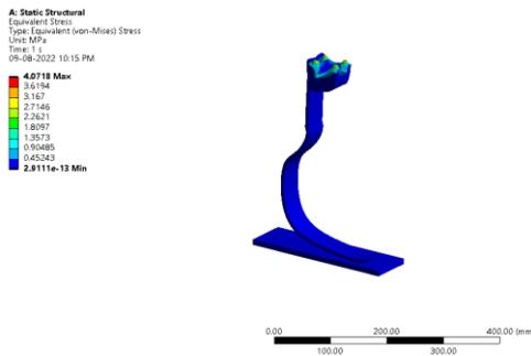
Figure 287: Equivalent Stress
