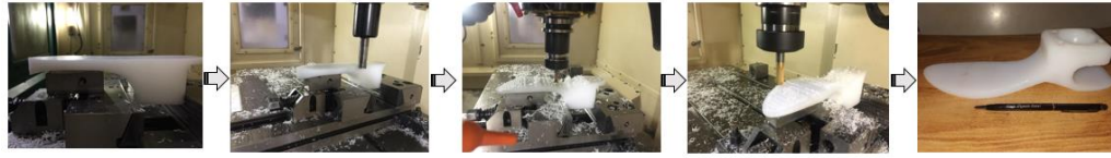
Figure 7.4: Machining process of prosthetic foot model
