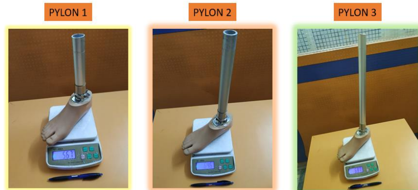
Figure 7.15: SACH Prosthetic Foot Structure with various pylon elements
