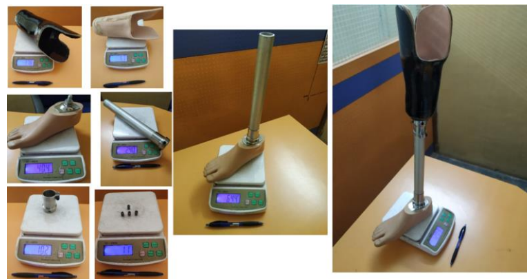
Figure 7.16: Weight for Novel prosthetic foot structure using pylon 2
