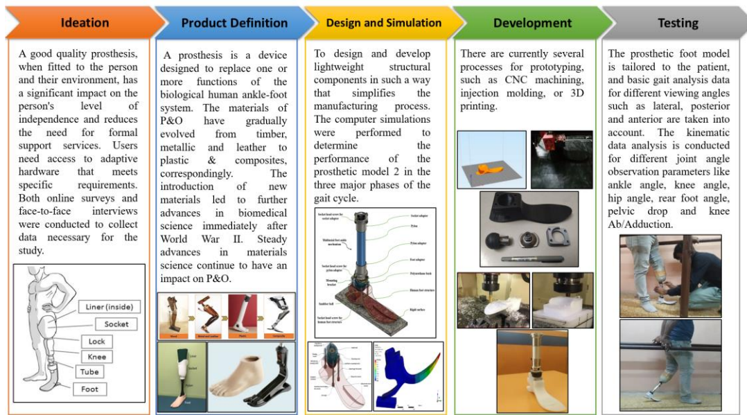
Figure 8.8: Development and testing process for novel prosthetic foot
