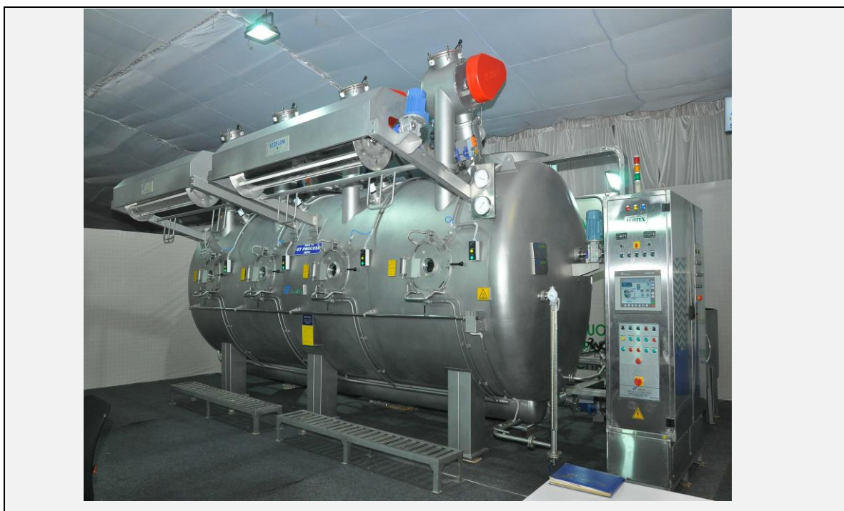
Figure 3.12 Ecotex Soft-flow dyeing machine (Ecotex- next generation engineering)
