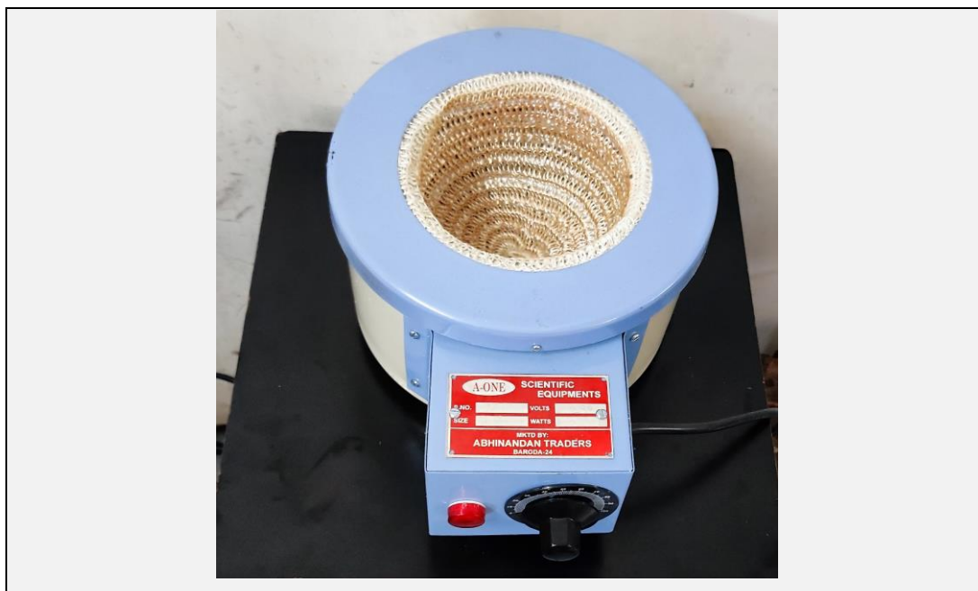
Figure 3.2 Electric heating mantle
