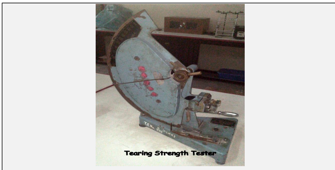
Figure 3.25 Elmendorf tear strength tester
