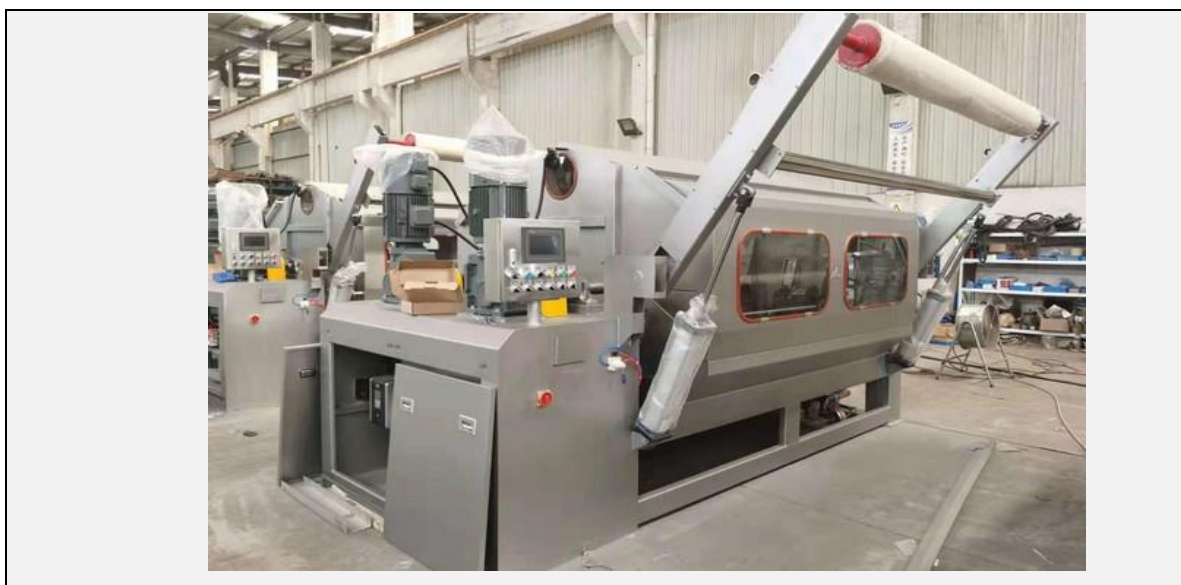
Figure 3.13 Closed Jigger machine (Mazharul, 2012)
