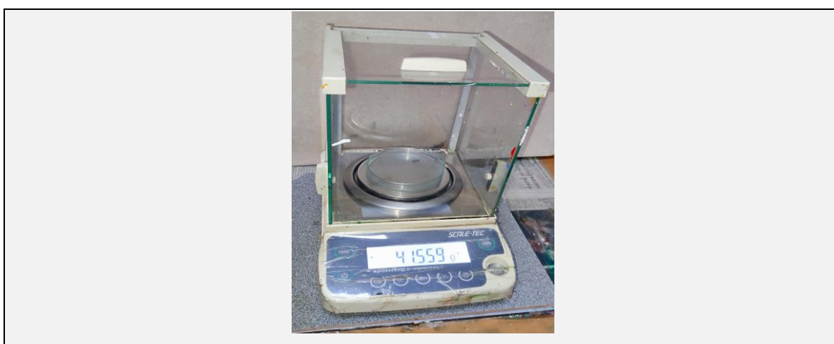
Figure 3.9 Petri-dish set up for solid content
