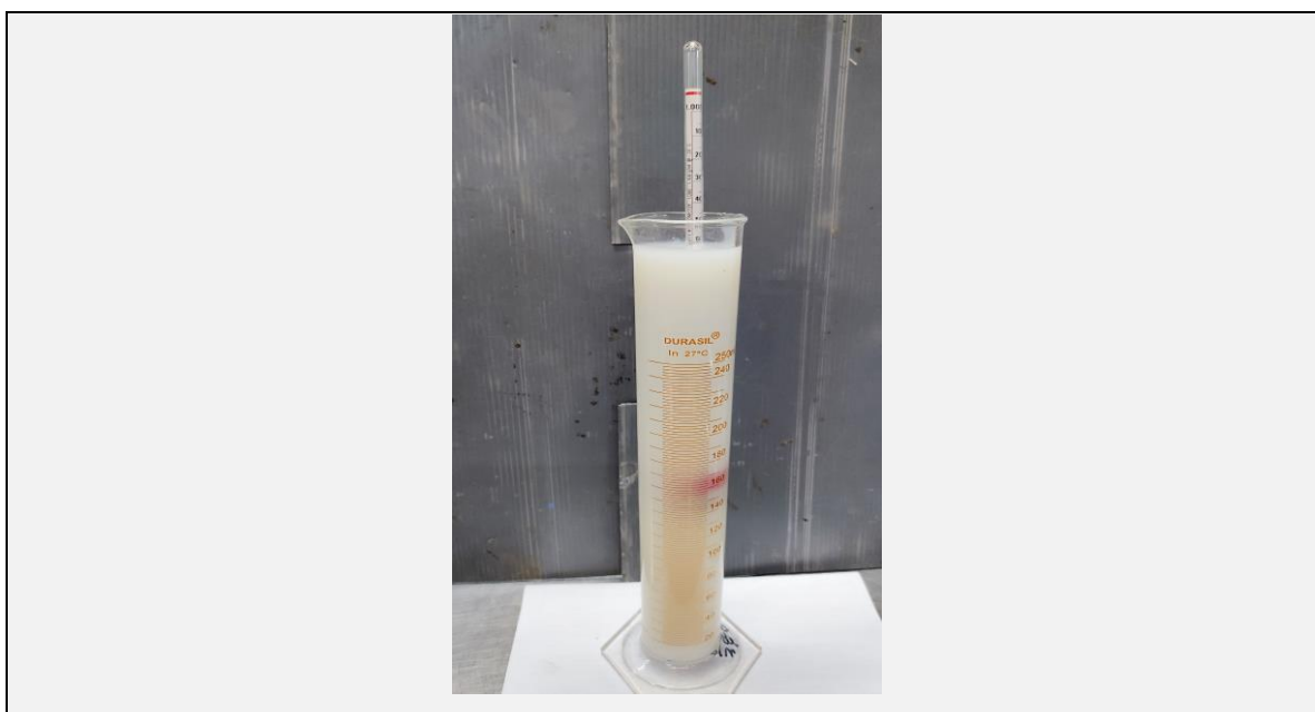
Figure 3.8 Hydrometer set up for specific gravity
