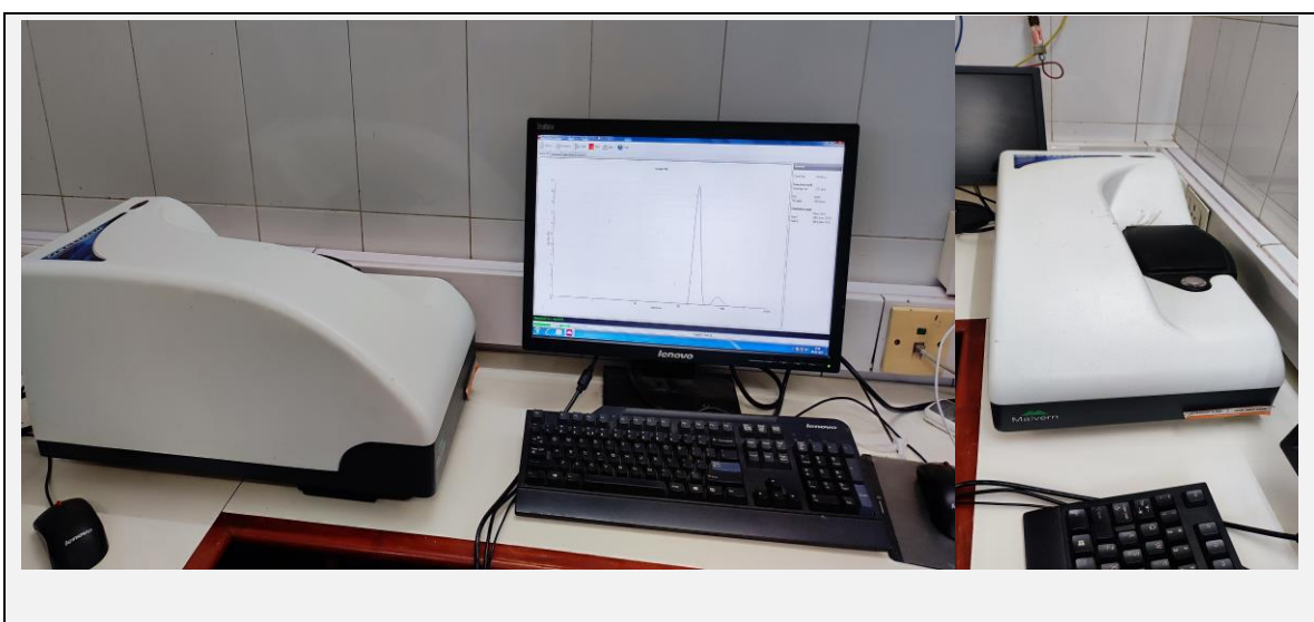
Figure 3.11 Malvern Particle Size Analyzer Set up
