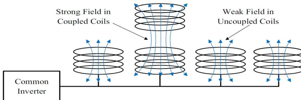
Figure 2-3 Dynamic charging systems with segmented-coil design for primary coil [27,30].
