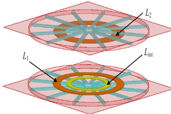
Figure 2-4 Coil with fixture.  $L_{int}$ = intermediate structure;  $L_1$ = primary coil structure;  $L_2$ = secondary coil structure [23].
