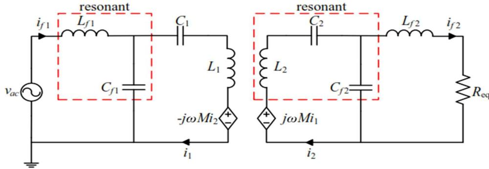
Figure 2-7 Two-sided LCC compensation.
