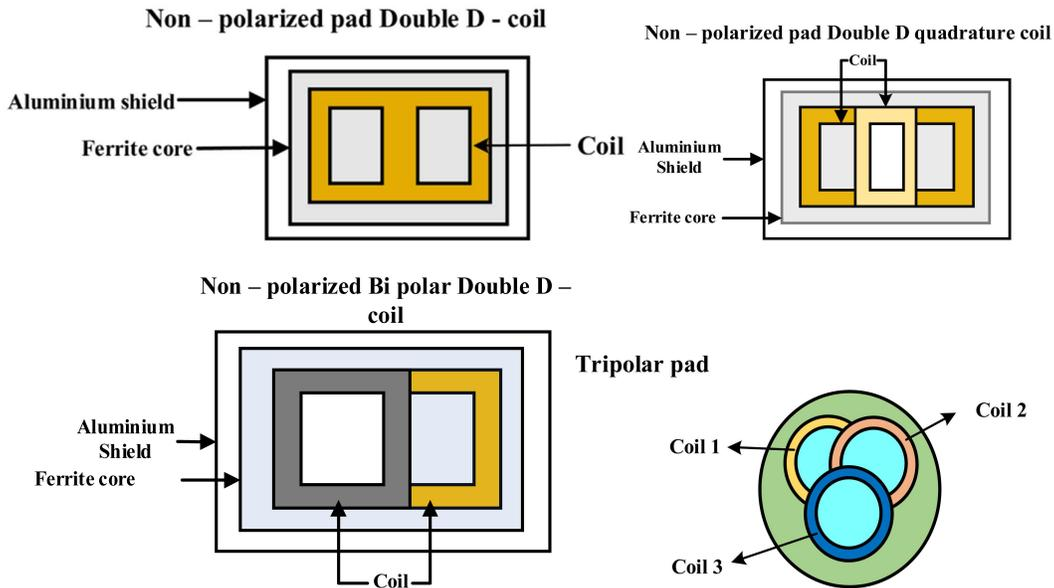
Figure 2-5 Different types of coil structures [104-106]
