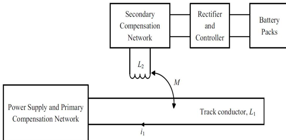
Figure 2-2 Dynamic charging systems with one coil design for primary coil  $L_1$  = track conductor;  $L_2$  = receiver coils;  $M$  = mutual inductance between  $L_1$  and  $L_2$ ;  $i_1$  = excitation for primary coil [27,30].
