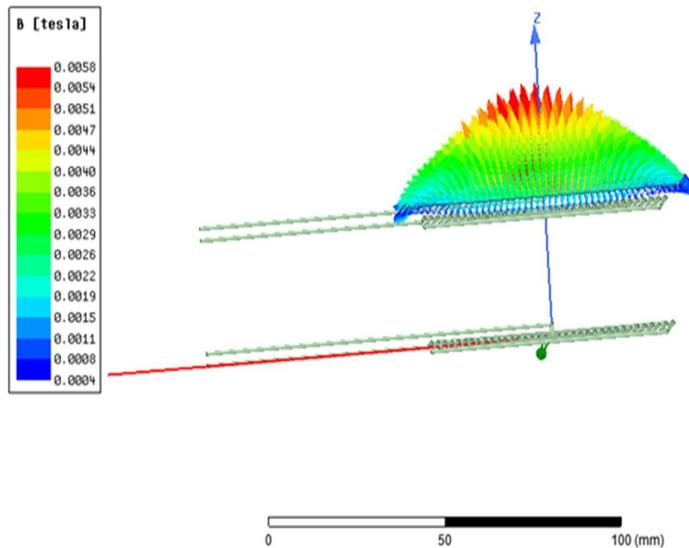
Figure 4-17 Flux density vector ZDist=30 mm and plate at 35 mm
