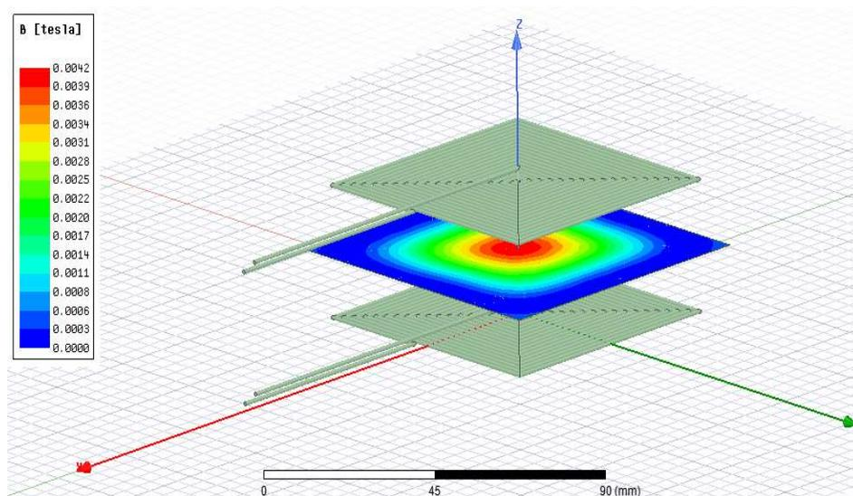
Figure 4-15 Flux density at ZDist = 30 mm.
