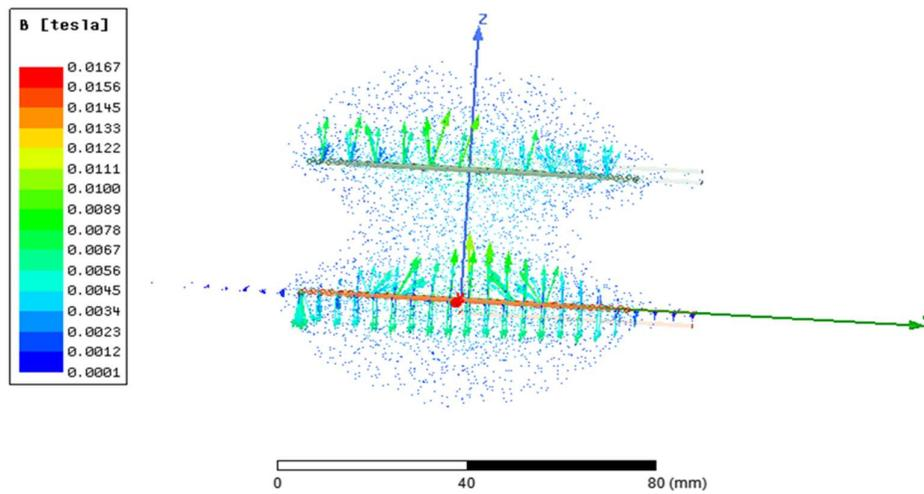
Figure 4-31 Flux density distribution around circular coils with less density setting.
