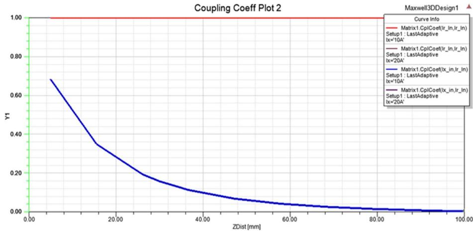
Figure 4-8 2D plot showing variation of k with ZDist (I = 10 & I induced = 20 Amps)
