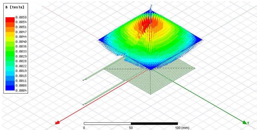
Figure 4-22 Flux density distribution at ZDist = 55 mm & plate 55 mm.
