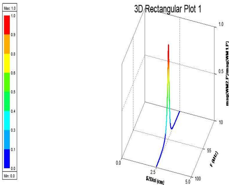
Figure 4-33 3D plot between f, ZDist and amplitude.
