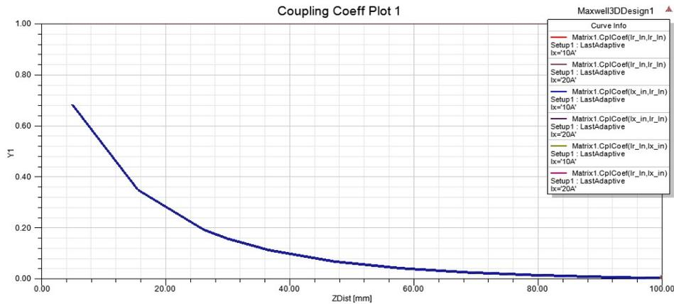
Figure 4-7 2D plot showing variation of  $k$  with ZDist ( $I = 10$  &  $20$  Amps)
