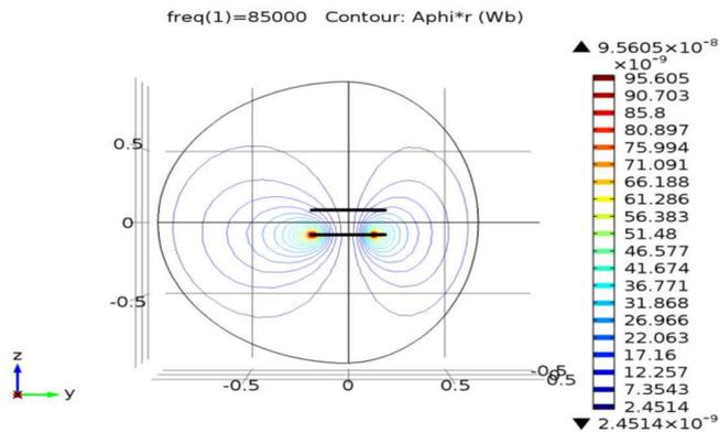
Figure 4-1 Magnetic flux lines of helix coil [ 7]
