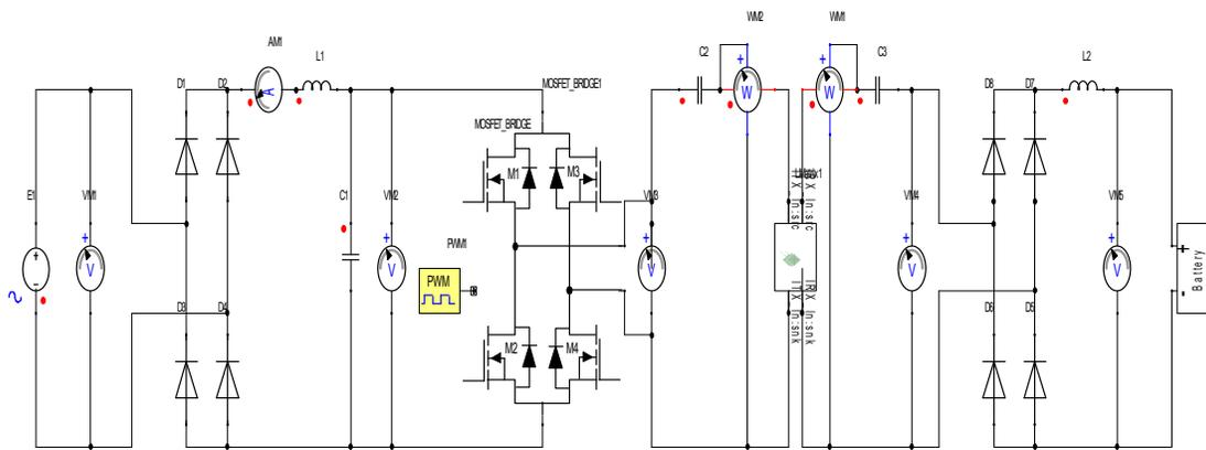
Figure 4-37 ANSYS Twin Builder circuit for circular geometry.
