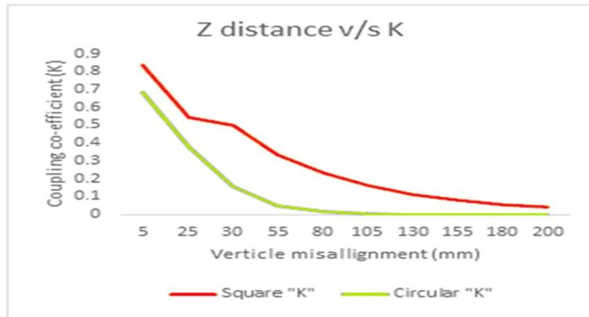
Figure 4-34 Comparative graph between ZDist vs Coupling coefficient.
