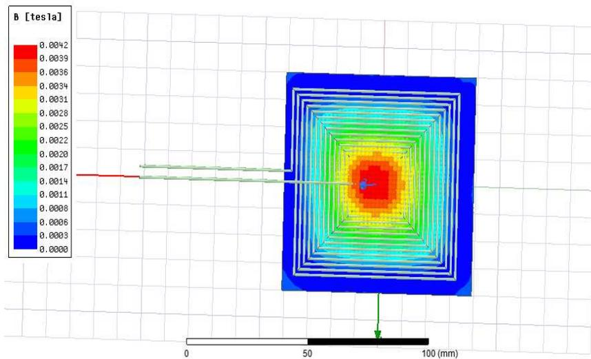
Figure 4-19 Flux density vector ZDist = 30 mm and plate at 15 mm top view.
