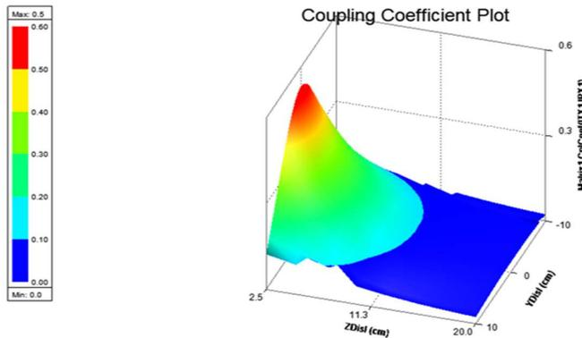
Figure 4-11 3D image showing variation of coupling co-efficient v/s YDist and v/s ZDist.
