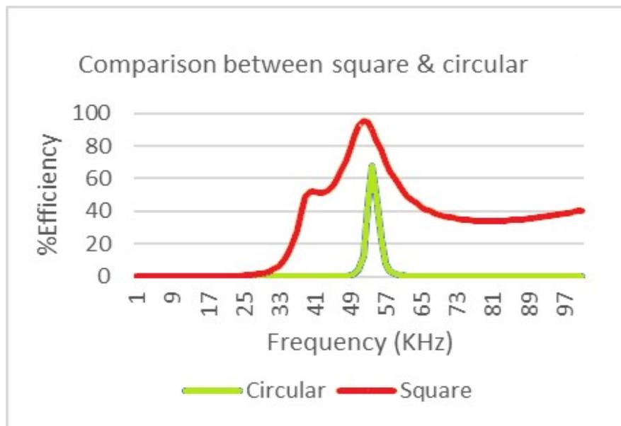
Figure 4-39 Comparison of efficiencies for square and circular coils.
