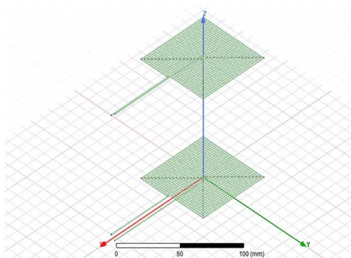
Figure 4-6 Design model of transmitting and receiving coil in ANSYS Electronics Desktop at ZDist of 150 mm
