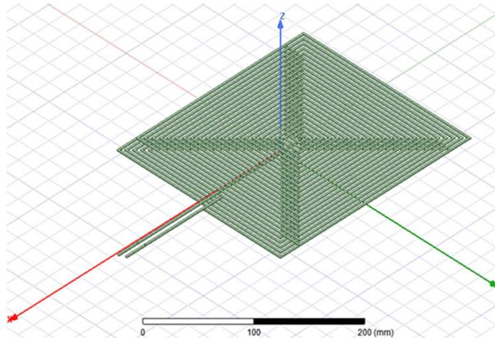
Figure 4-5 Design model of transmitting and receiving coil in ANSYS Electronics Desktop at ZDist of 5 mm
