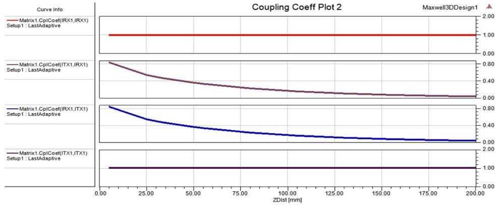
Figure 4-24 Variation of coupling coefficient with respect to ZDist for circular coil
