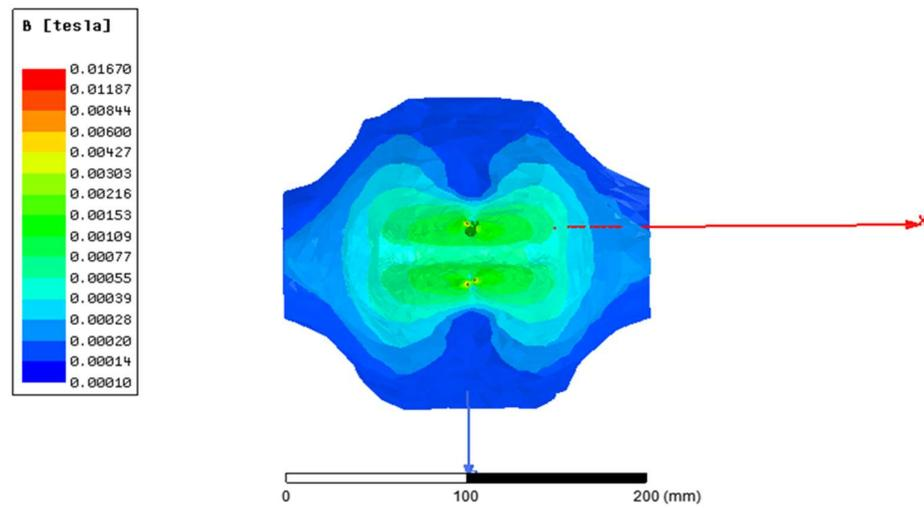
Figure 4-32 Flux density distribution around circular coils in cloud form.
