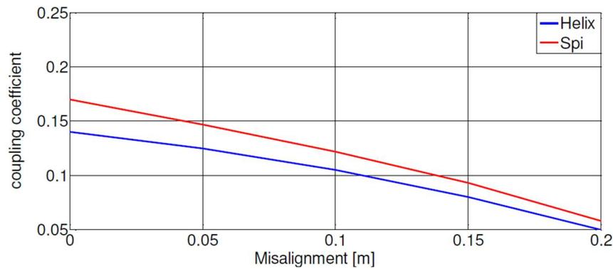
Figure 4-4 Variation of k with z axis misalignment for helix and spiral coils
