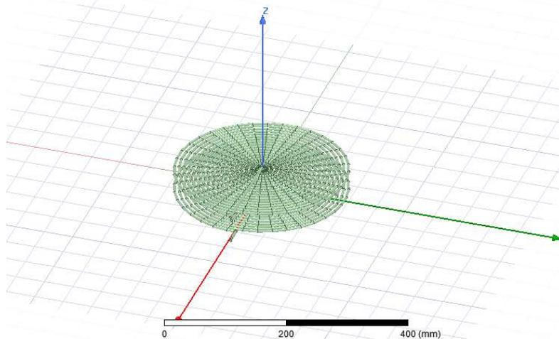
Figure 4-23 Circular coil configuration at ZDist = 5 mm
