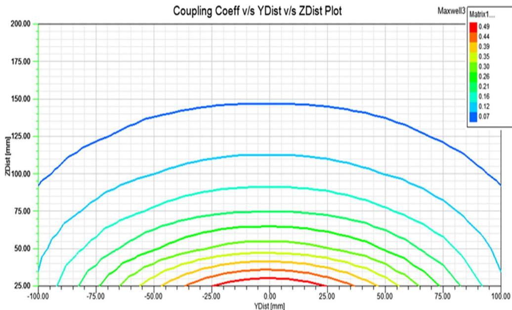
Figure 4-12 Contour of coupling co-efficient for YDist and ZDist
