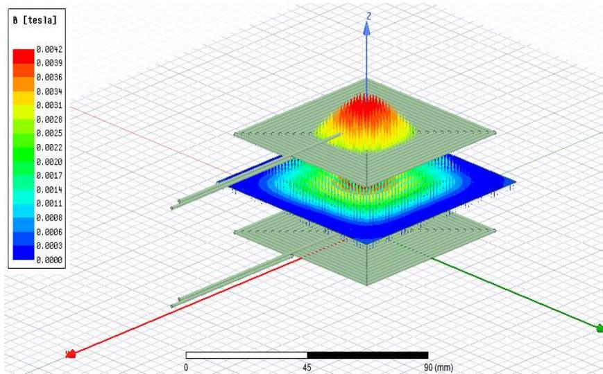
Figure 4-16 Flux density vector at ZDist=30mm.
