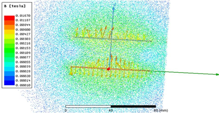
Figure 4-30 Flux density distribution around circular coils.
