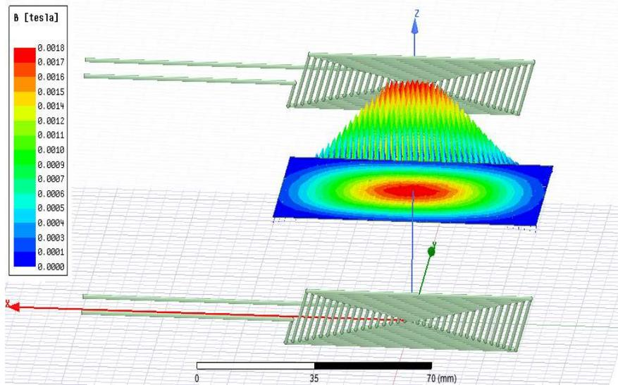
Figure 4-21 Flux density distribution at ZDist = 55 mm & plate 30 mm.
