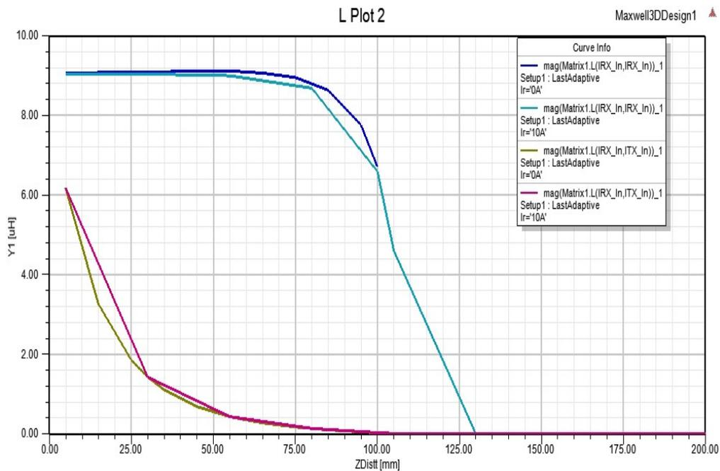
Figure 4-13 Plot of L<sub>1</sub> v/s ZDist, L<sub>2</sub> v/s ZDist & M<sub>12</sub> v/s ZDist (0 Amp & 10 Amps)
