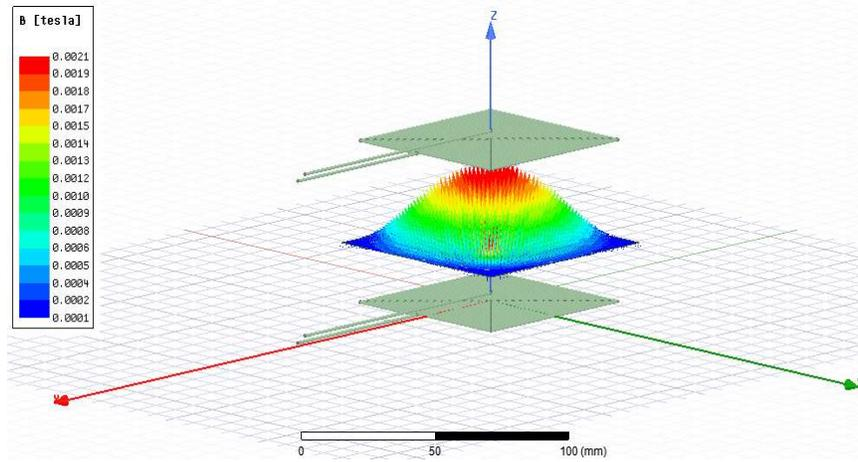
Figure 4-20 Flux density distribution at ZDist = 55 mm & plate 20 mm.
