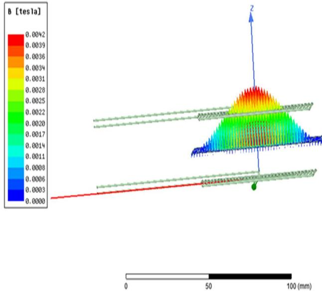
Figure 4-18 Flux density vector ZDist=30 mm and plate at 15 mm.
