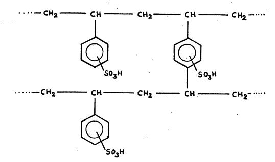
For very low crosslinked resins the bridging of aromatic rings through sulfone can occur by electrophilic ring substitution mechanism.
