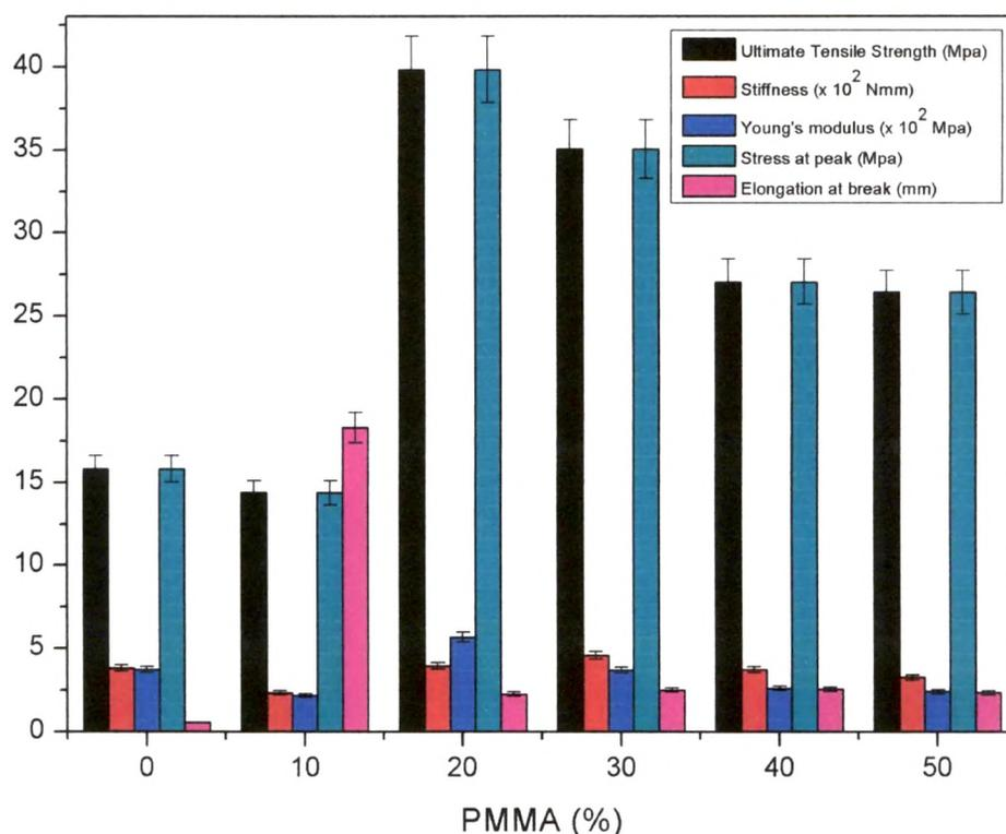
**Figure 3.4** Variation in Ultimate tensile strength, Stiffness, Young's Modulus, stress at peak, Elongation at break, as a function of PMMA content
