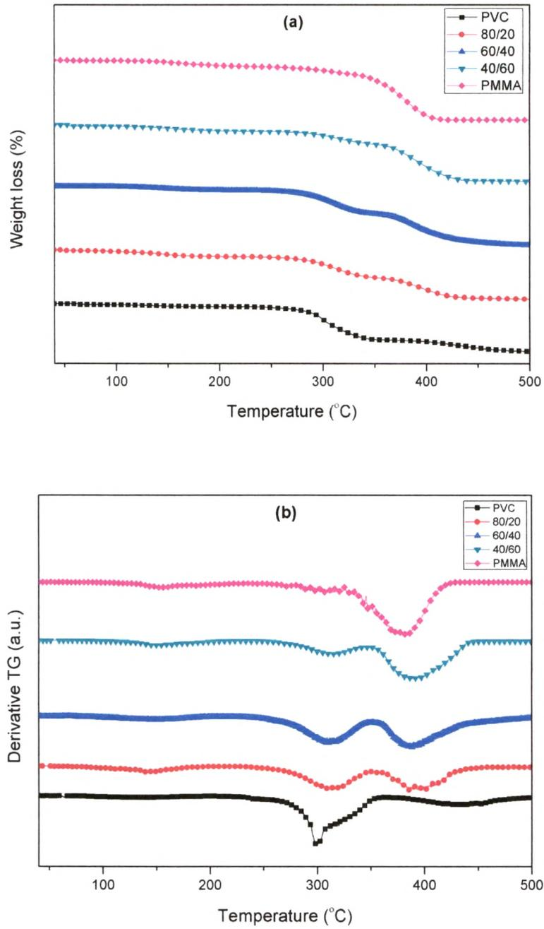
Figure 3.5 (a) TG of pure PVC, pure PMMA and their blends (b) Derivative TG of pure PVC, pure PMMA and their blends
