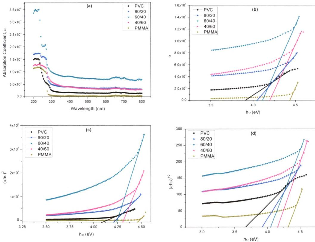
**Figure 3.2** Plot of (a) Absorption coefficient ( $\alpha$ ) vs Wavelength ( $\lambda$ ), (b) Absorption coefficient ( $\alpha$ ) vs Photon Energy ( $h\nu$ ), (c)  $(\alpha h\nu)^2$  vs  $h\nu$ , (d)  $(\alpha h\nu)^{1/2}$  vs  $h\nu$
