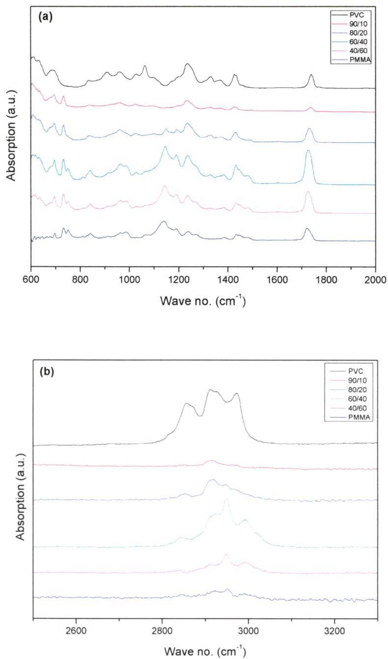
Figure 3.1 FTIR Spectra of pure PVC, pure PMMA and Their blends (a) in the range 600 – 2000  $\text{cm}^{-1}$  (b) in the range 2500 – 3300  $\text{cm}^{-1}$
