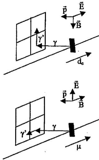
Figure 4.5: Compton scattering in a Clover detector for stretched electric (top panel) and magnetic (bottom panel) dipole transition.
