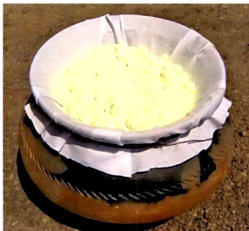
Fig. 3.11. Picture depicting the purification of sulphur.
