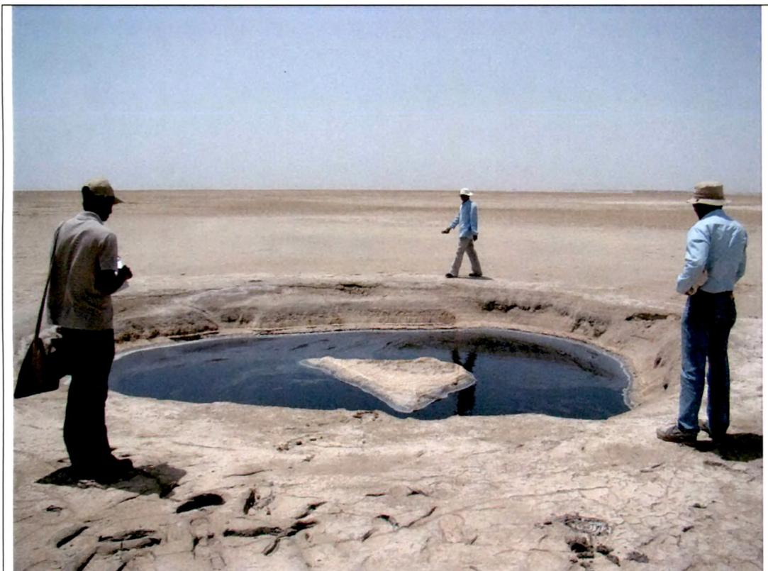
*Fig. 5.1: Liquefaction crater seen in epicentral area of 2001 Bhuj earthquake.*
