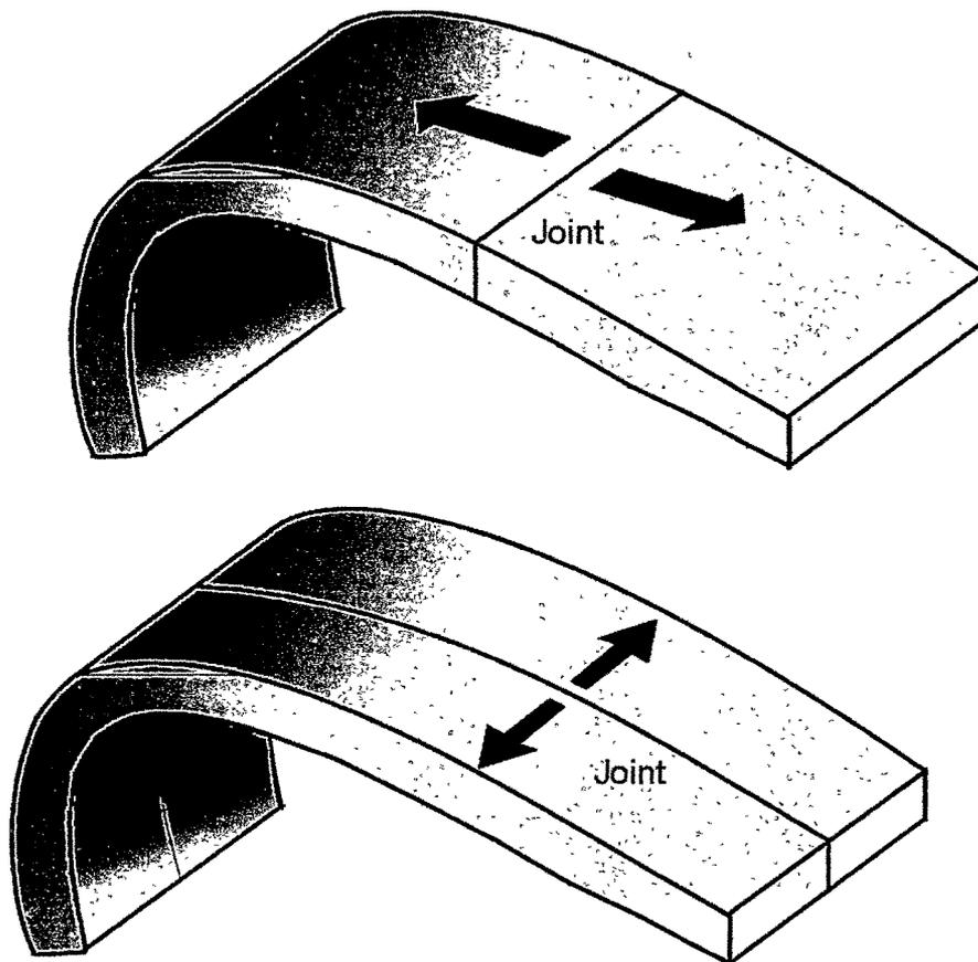
**Fig 4.40 Formation of different joints sets, i.e. one perpendicular to the hinge of the fold and the other parallel to it (after Hancock, 1985)**
