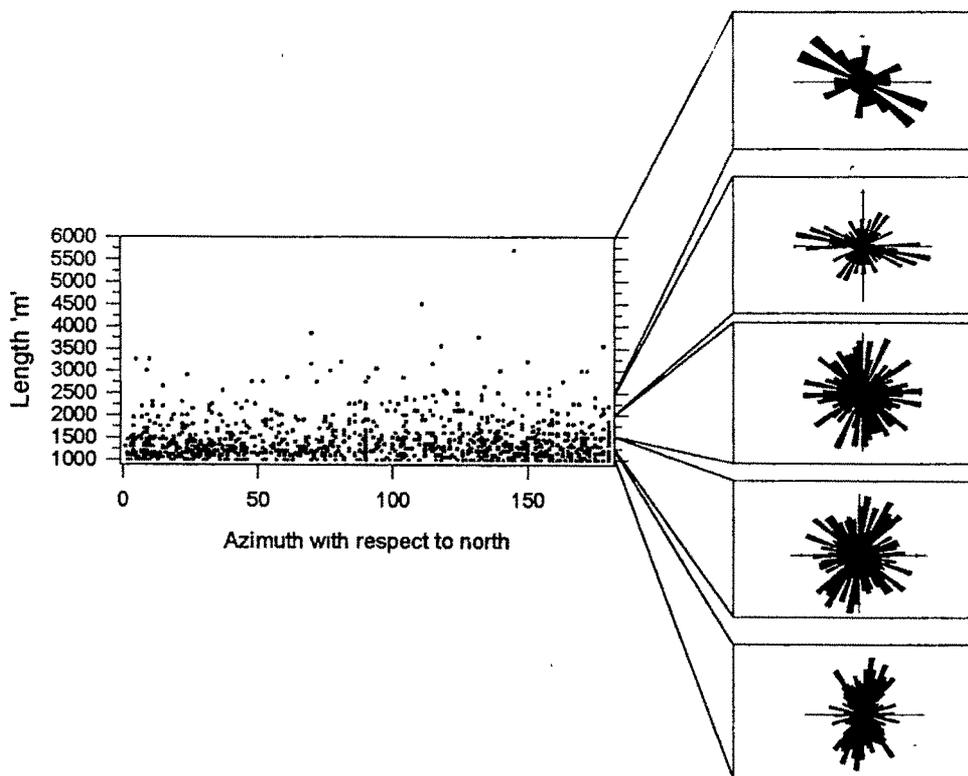
**Fig 4.46 Graph showing the Length-Azimuth relationship of the lineaments**
