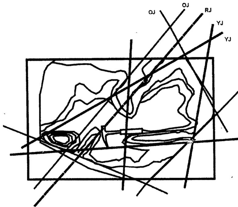
**Fig 4.44b** A line drawing showing the superimposition of subsequent joint sets responsible for the modification of the preexisting structures (OJ – older joint polygon, RJ – a joint set showing no signs of weathering, which is seen to cut through the compound structures and hence considered to have developed in recent times, YJ – a joint polygon responsible for the modification of the already existing structures which is subsequent to OJ but has formed prior to RJ)
