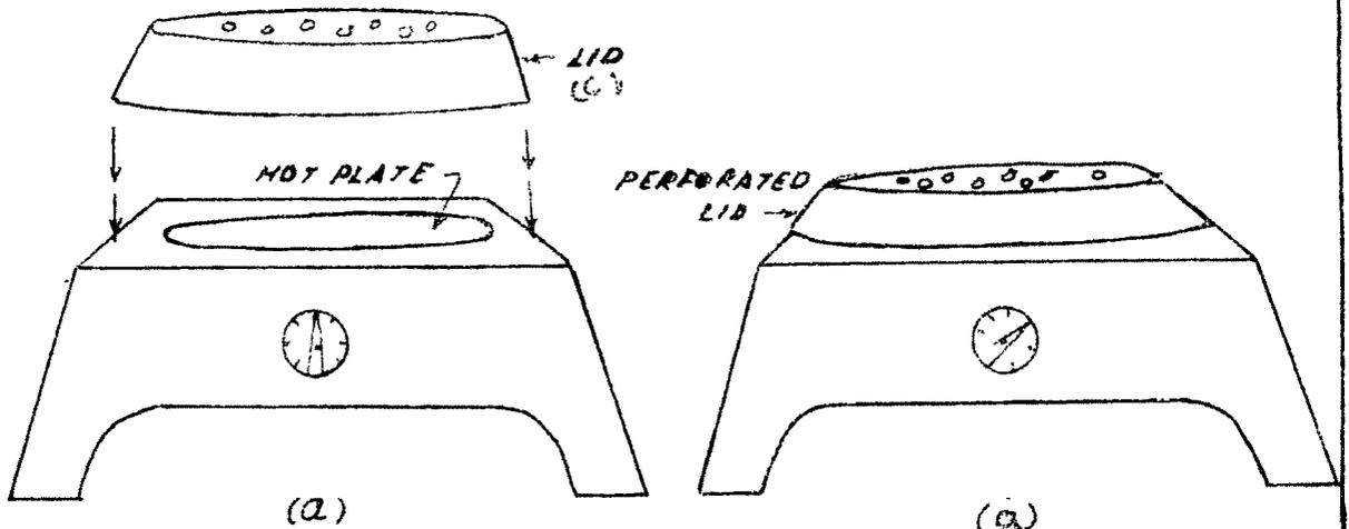
POSITION OF PERFORATED LID ON HOT PLATE
