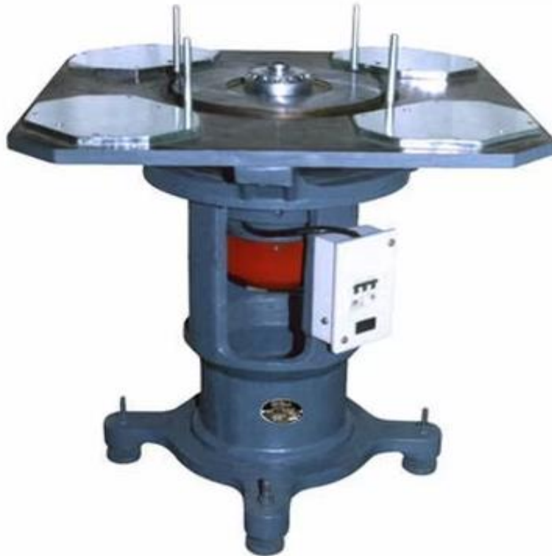
Plate 5: Diamond Polishing Machine (27)
