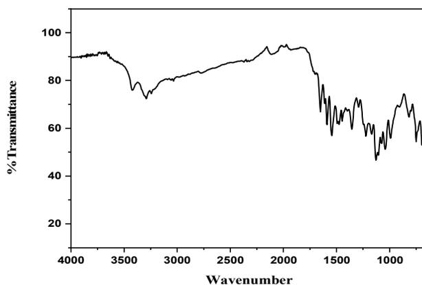
**Figure 17:** IR spectra of reactive dye Z33
