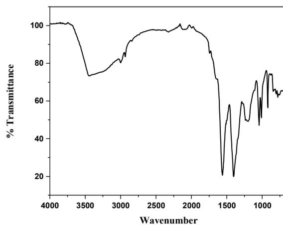
Figure:18 IR spectra of reactive dye Z49
