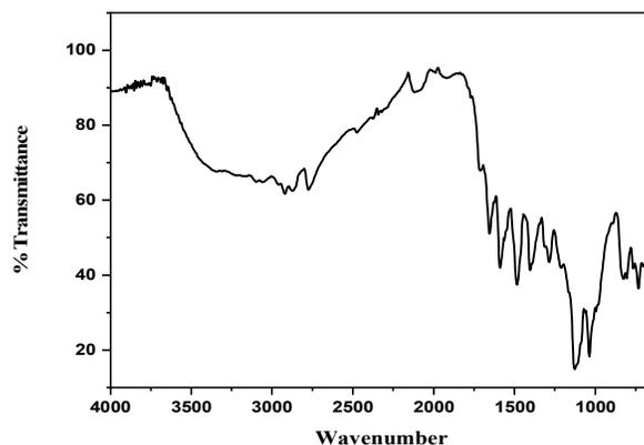
**Figure:19** IR spectra of reactive dye Z53
