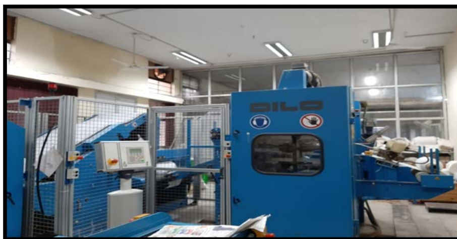
Plate 3.14: Needle-punching machine (laboratory at IIT Delhi)
