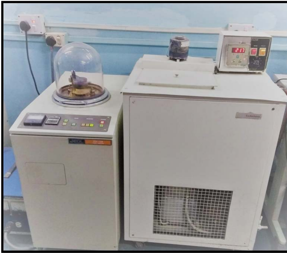
Plate 3.3: Sample preparation unit for SEM testing in BTRA laboratory
