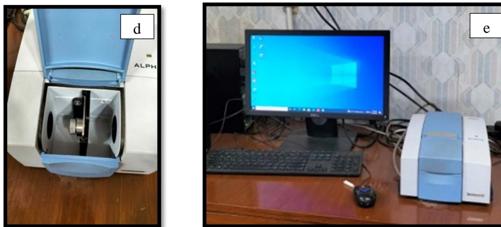
Plate 3.13: FTIR Setup (a) Sample preparation (b) Hydraulic pellet press (c) KBr pellet (d) Sample holder (e) Setup for spectra graph
