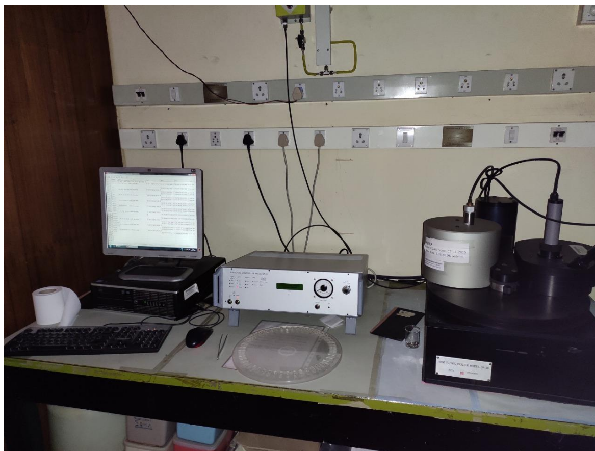
Figure 2.7 Risø TL/OSL reader DA 15 (Bøtter-Jensen et al., 2003) instrument.
