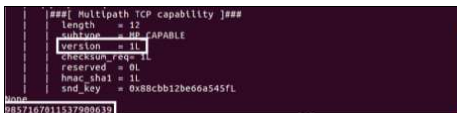
Figure 11 Extracting keys captured during initial handshake to perform ADD_ADDR attack by using python script
