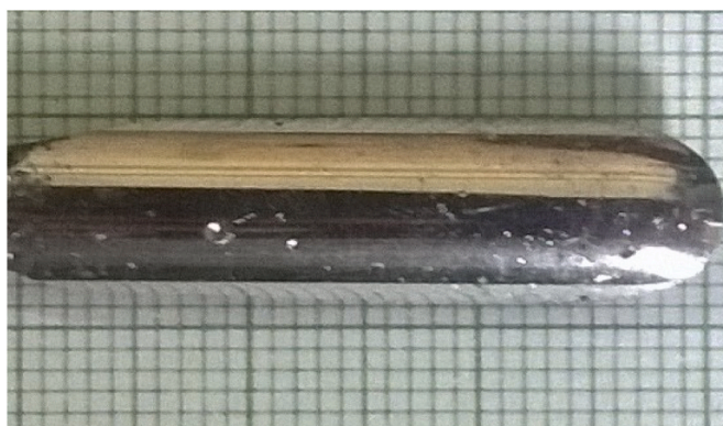
Fig. 2. As grown crystals of \text{InBi}_{0.90}\text{Te}_{0.10} .
