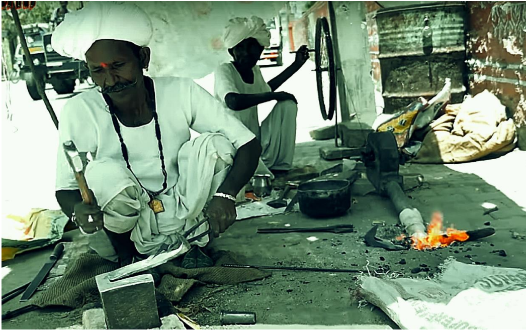
Plate 4.2 A traditional Blacksmith ( Lovār ) crafting Spade ( Fāvaḍā ) at the Bhīnmāl city, Rājasthān .
