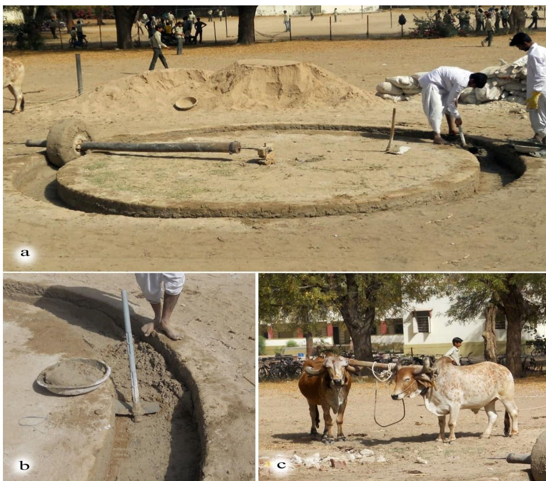
Plate 4.18 (a) Ghaṭa (traditional stone wheel lime crusher), (b) Crushed lime (c) The pair of Ox used to twiddle Ghaṭa .
