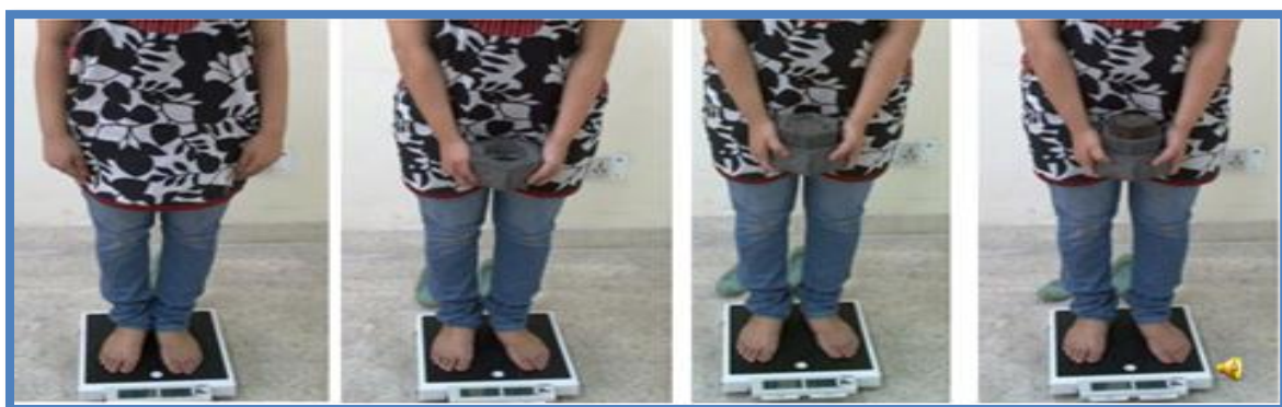
Plate 4.17: Testing sensitivity of balances (adult + standard weight)
