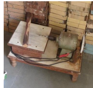
Plate 4.7: Drill machine used for drilling air holes in wood block
