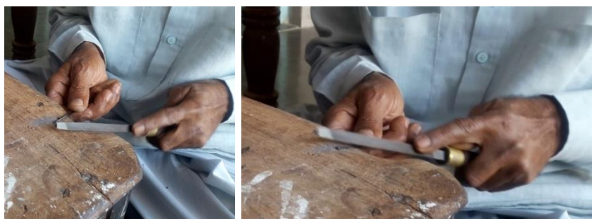
Plate 4.63: Step 3-Filing was done to acquire desired shape of chisel
