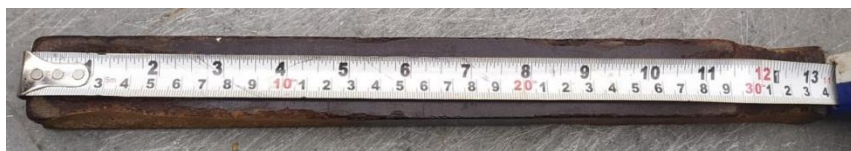
Plate 4.89: Mallet - A tool used to tap on chisel while carving
