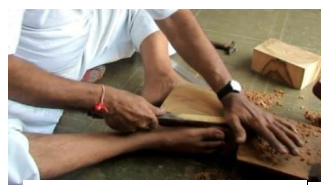
Plate 4.10: Finishing of wood piece using file
