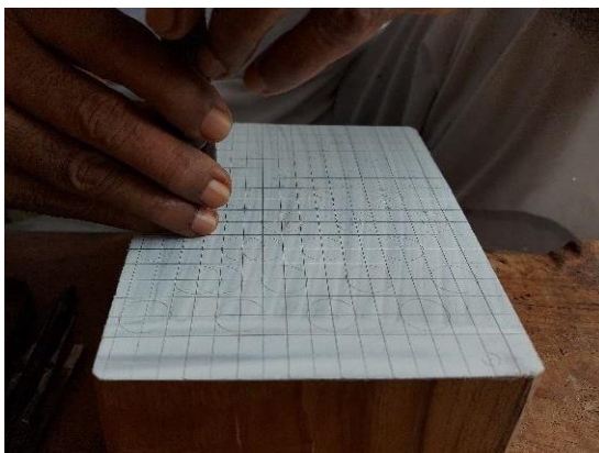
Plate 4.15: Drawing the design directly on wood piece
