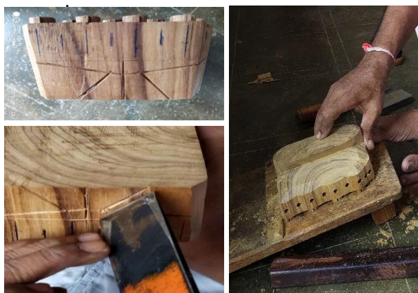
Plate 4.24: Stages of carving out a handle from the wood block with carved design – Marking, Eliminating and Finishing
