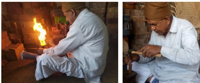
Plate 4.61: Step 1 - Turning on the stove and fixing the rib into the wood
