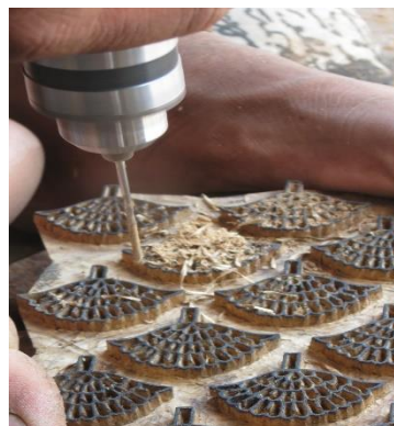
Plate 4.23: Drilling air holes using electric hand drill
