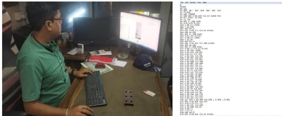
Plate 4.97: Programme generated in CNC friendly programming language (G-code)
