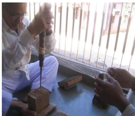
Plate 4.22: Making air holes in wood block manually Source: Trivedi 2011, unpublished master's
