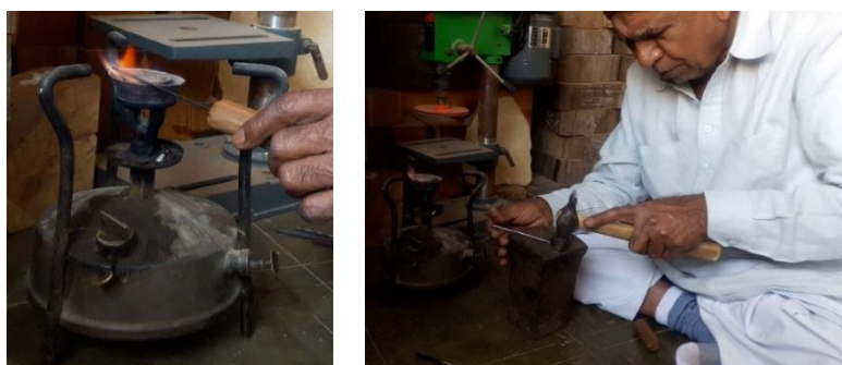
Plate 4.62: Step 2 - Heating the umbrella rib and making it flat by hammering
