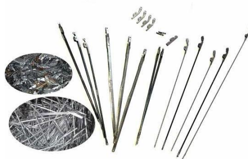
Plate 4.60: Umbrella ribs of different gauges used in making chisels
