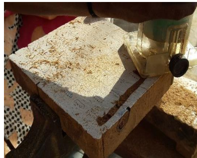
Plate 4.20: Removing excess wood using grinder
