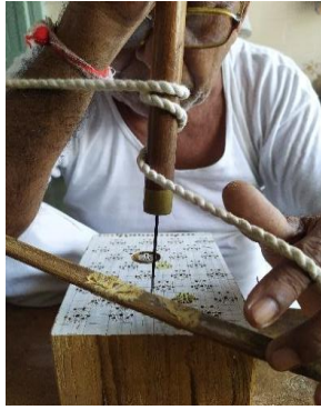
Plate 4.17: Drilling holes in negative area of the design
