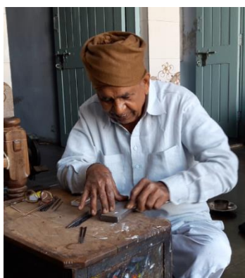
Plate 4.65: Step 5- Sharpening the chisel using emery stone
