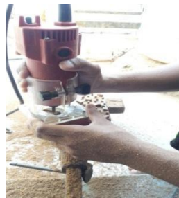
Plate 4.6: Trimmer used for removing negative area from filling block
