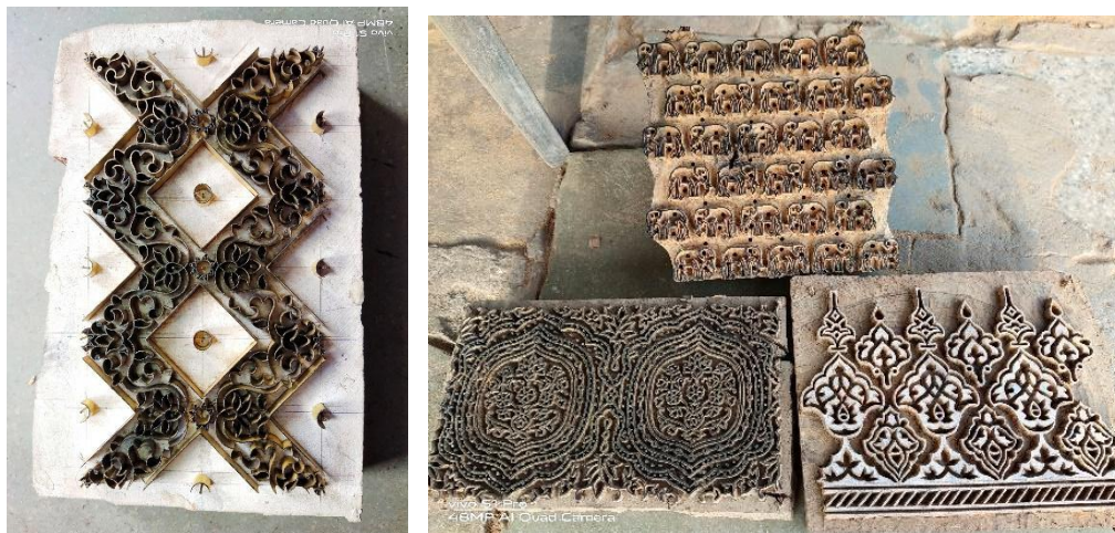
Plate 4.58: Metal blocks (Left) and Wood blocks (Right) prepared by block makers of Farukhabad, Ahmedabad workshop
