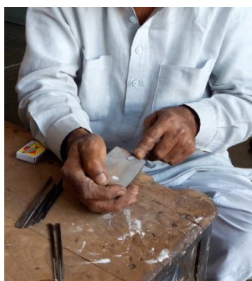
Plate 4.65: Step 5- Sharpening the chisel using emery stone
