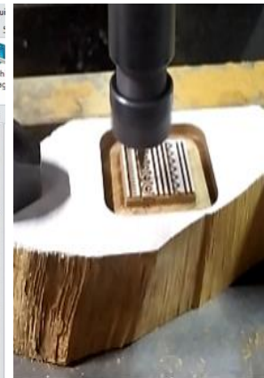
Plate 4.101: Carving process done by VMC machine
