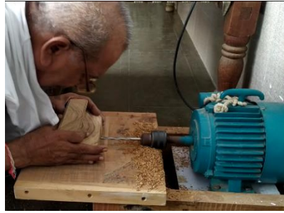
b. Craftsmen using trimmer and amount of wood dust produced
