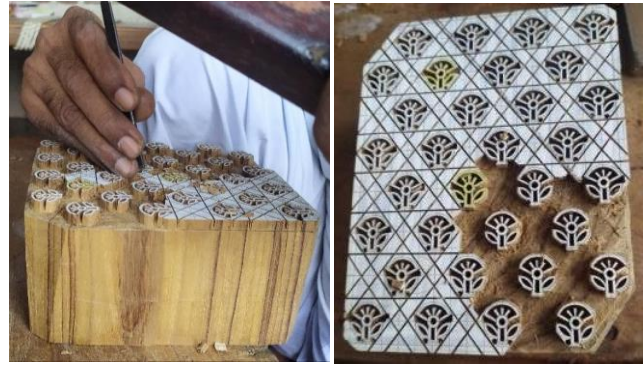
Plate 4.18: Breaking holes and clearing the base
