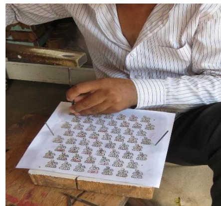
Plate 4.16: Transferring the design onto wood piece by tracing from the imprint
