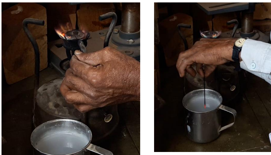
Plate 4.64: Step 4 - Heat up the chisel on a high temperature till it turned red and cold down immediately
