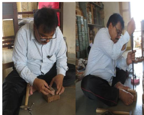
Plate 4.25: Attachment of handle separately on to the carved block
