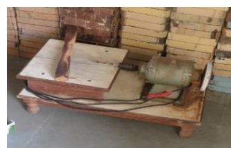
f. Drill machine: used dill air holes in wood
