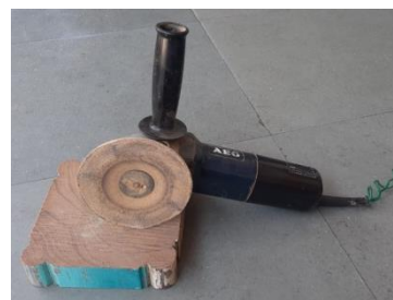
Figure 4.6: Finishing of wood piece using electric grinder
