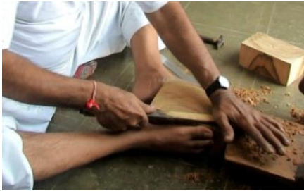
c. Leveling and polishing of wood piece using file
