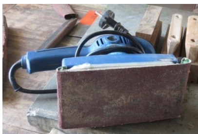
Figure 4.6: Finishing of wood piece using electric grinder
