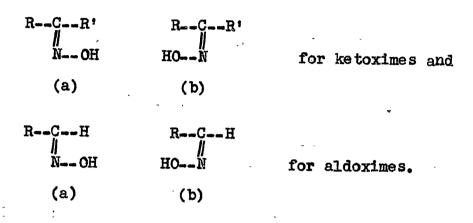
Hantzsch' method of orienting aldoximes depended on the fact that an acetyl derivative of one isomer regenerated a parent oxime on treatment with an alkali, whilst an acetyl derivative of the other lost acetic acid producing a nitrile. He assumed that the elimination of acetic acid took place from cis and not from the trans isomer. Similarly, a structure to the ketoximes was ascribed on the basis of Beckmann rearrangement wherein cis-interchange of radicals was assumed to take place.
