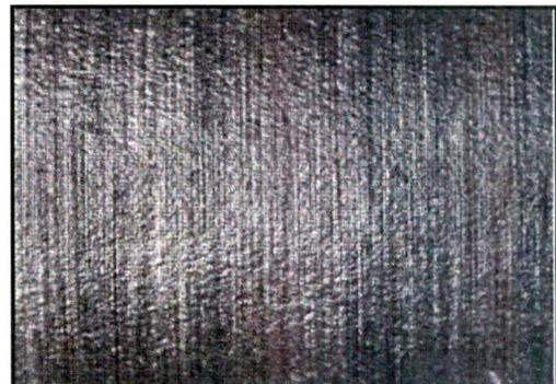
**Fig.2.53** Passing Test Specimen (View the Bend Area 20X)
