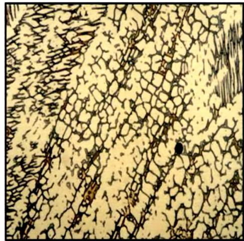
Fig, 2.25 FA mode weld metal in 312 austenitic stainless steel
