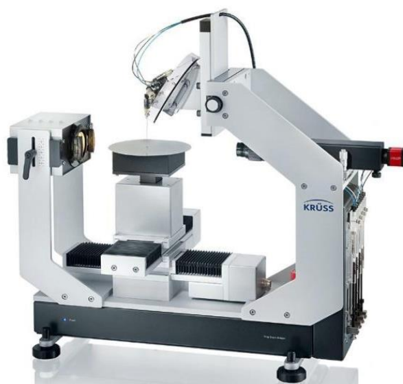
Figure 2.10: Contact angle instrument (Krüss DSA100 contact angle goniometer, Germany) used for the present work
