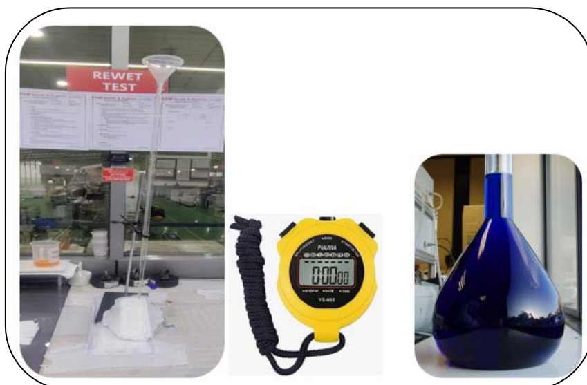
Fig. 3.55 Absorption and rewet instrument for sanitary napkins
