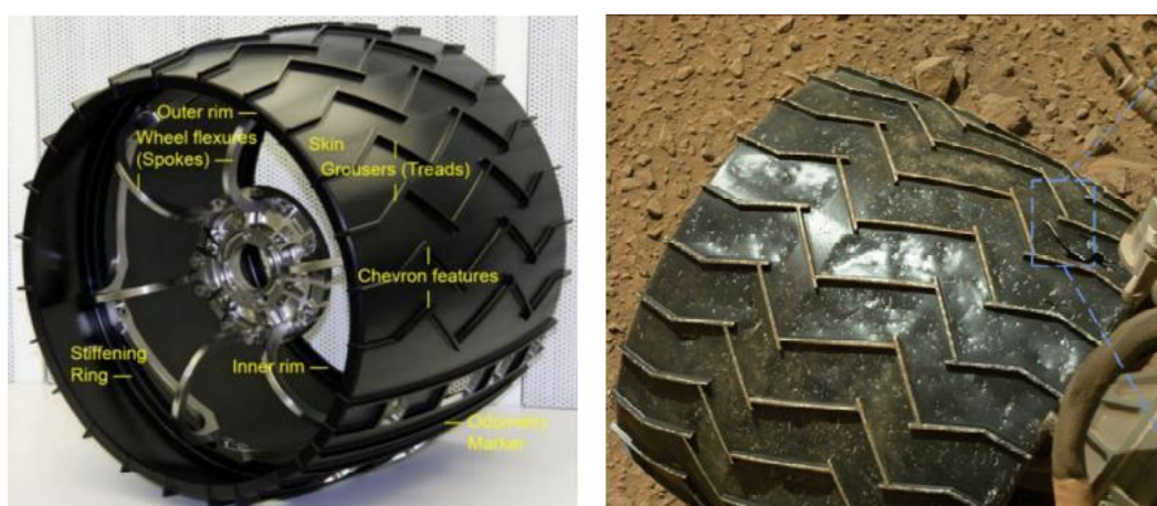
Figure 1.5 Curiosity rover wheels of 7075-T7351; a) on the ground, b) under operation conditions on Mars [13].
