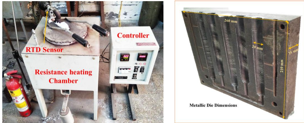
Figure 3 Experimental set-up for melting Al7075 (left), and metallic die with dimensions to pour liquid melt.
