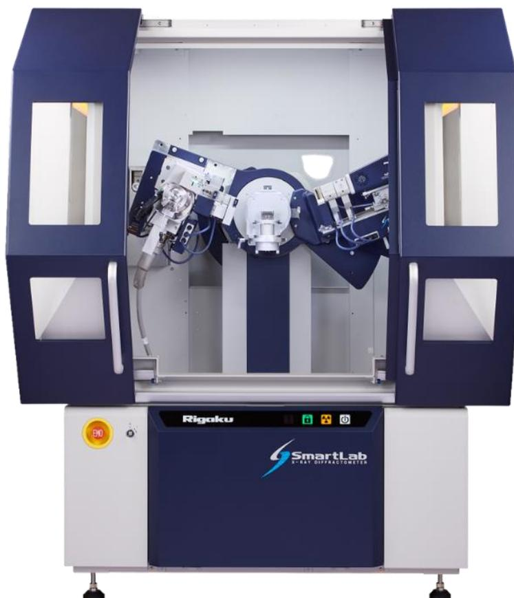
**Figure 2.10:** X-ray diffraction instrument (smartLab SE)
