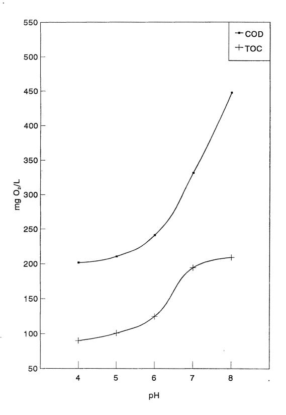
Fig.7. COD values of oil waste water after treatment with different concentrations of FeCl<sub>3</sub> at varying pH
