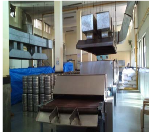
Chapati (Roti) making Machine produces 50,000 Chapatis in an hour
